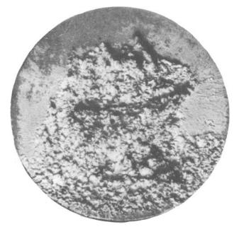
FIG. 3-Example of the lead specimen surface damaged totally.
