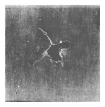
FIG. 8-Typical failure of elastomeric specimen from water gun test.
