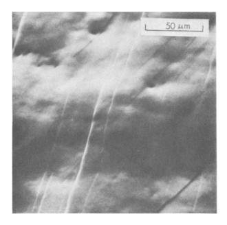
FIG. 4a—Multiple slip on the {110} single-crystal surface after 5 s of erosion.
