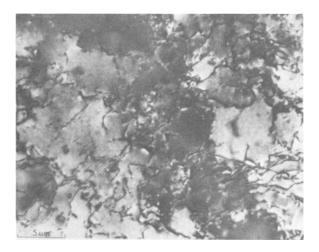
FIG. 9a—TEM of polycrystalline aluminum after 5 s of erosion at an amplitude of 43  $\mu m$ .
