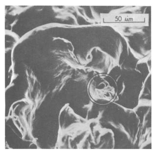
FIG. 4c—Development of crater after 82 s of erosion on the {110} surface of aluminum single crystal. Material loss has occurred from the circled area.
