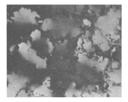
FIG. 13—Cell structure in polycrystalline aluminum rolled 5 per cent at room temperature.
