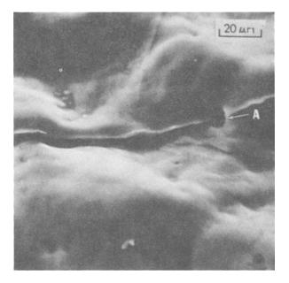
FIG. 8a—Grain boundary pulled apart after 15 s of erosion in bicrystal No. 3. The pit labelled A is typical of those considered to be caused by the collapse of a single bubble.
