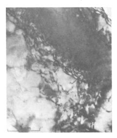
FIG. 10—TEM of polycrystalline aluminum after 30 s of erosion at an amplitude of 88  $\mu$ m.
