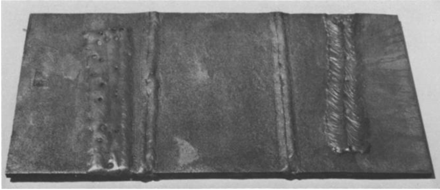
FIG. 17—Welded ASTM-A-514 (T-1) structural steel specimen with weld third-face deposits. Although corrosion attack appears relatively uniform, the thickness variation was 0.043 in.
