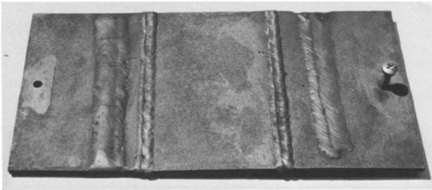
FIG. 18—Welded cathodically protected (zinc anodes) ASTM-A-514 (T-1) structural steel specimen with two 1 by 5-in. weld hard-face deposits to extreme left and right. Corrosion attack resulted in 0.027-in. thickness variation.
