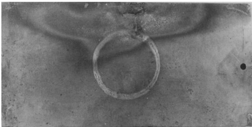
FIG. 26—Specimen 21—maraging stainless steel (Almar 362) heat-treated to H1050 condition, welded without filler metal. Pitting and crevice corrosion has perforated 0.050 sheet at weld edge of sheet.
