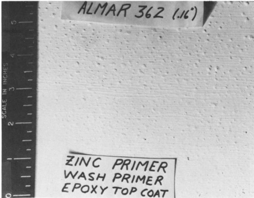
FIG. 9—Closeup of typical blistering that occurred on specimens coated with Systems 2 and 3 (Table 5).
