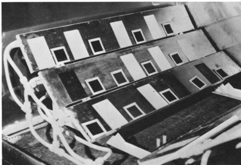
FIG. 3—Chamber chill racks.
