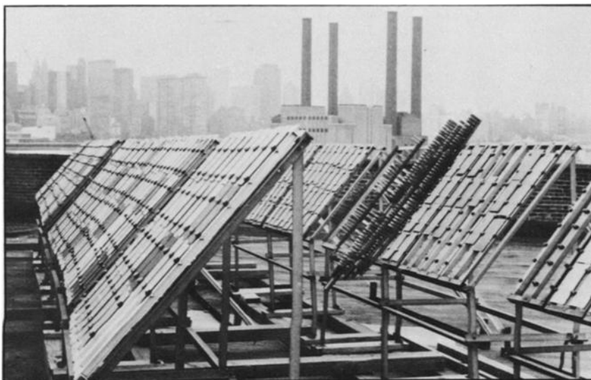
FIG. 2— Atmospheric corrosion racks, stands, and panels at the Brooklyn, N.Y. test site.
