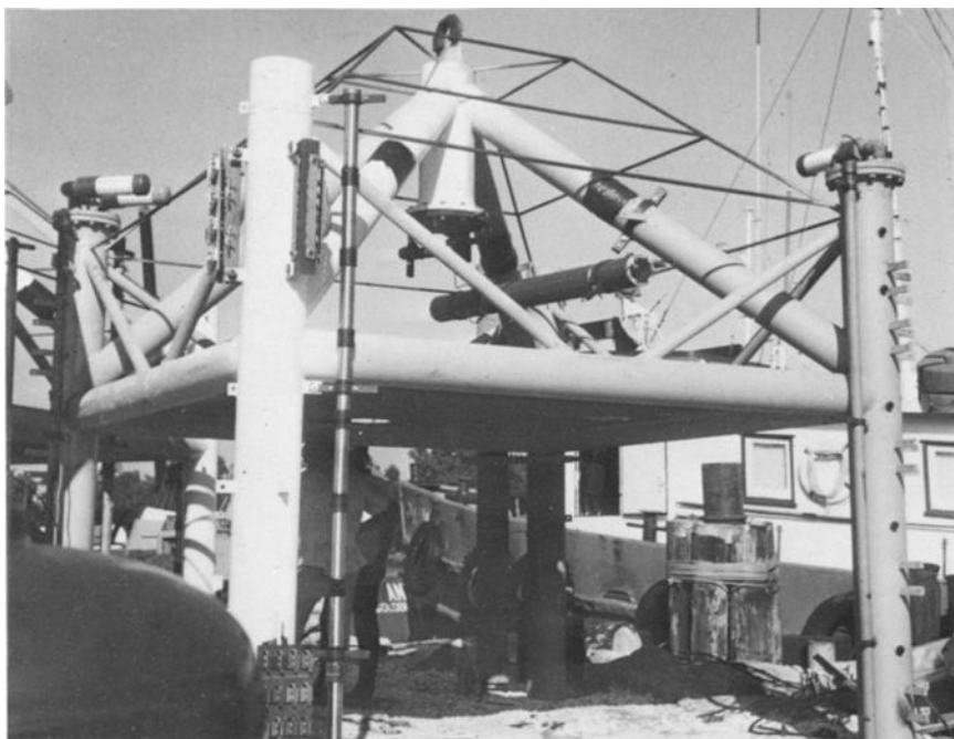
FIG. 5—Deepwater corrosion test rack just prior to launching in West Delta Block 134 Field.
