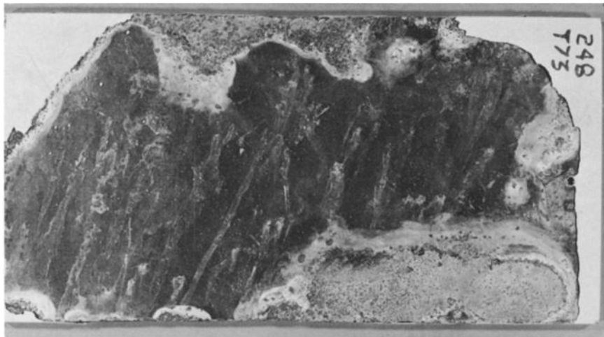
FIG. 25—Specimen 248—aluminum alloy 7075-T73 coated with zinc-rich primer (Zinc-Lock), wash primer, and epoxy topcoat. Coating system did not adhere, resulting in extensive pitting corrosion.
