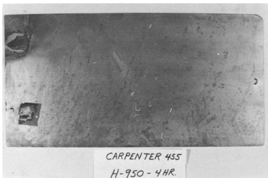
FIG. 12—Crevice corrosion (top left) that occurred under adhesive tape on Carpenter 455 stainless steel specimens.
