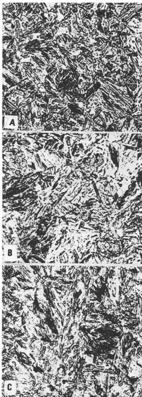
FIG. 1—Typical microstructure of high-hardness armor steels. Etchant: Picral ( \times 1000 ).
