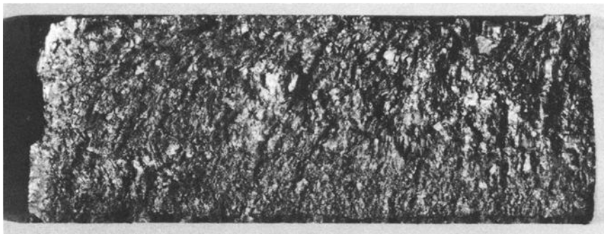
FIG.1— Photograph of failed specimen CT-7 (×6).
