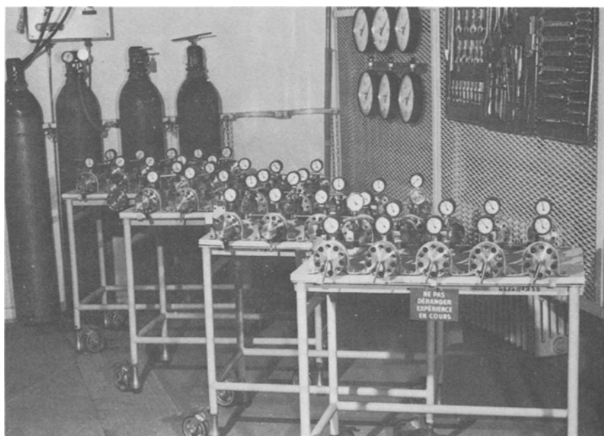
FIG. 10—Delayed failure racks.
