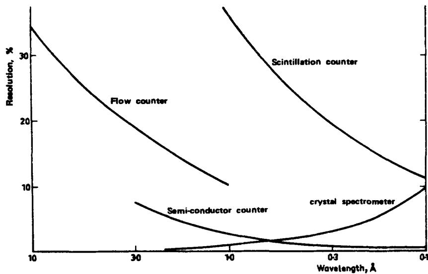
Comparative resolutions of the flow counter, the scintillation counter, the semiconductor counter, and the crystal spectrometer.
