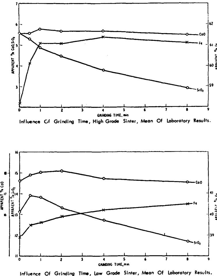
Fig. 2 Effect Of Grinding Time on XRF Analysis Of Sinters.
