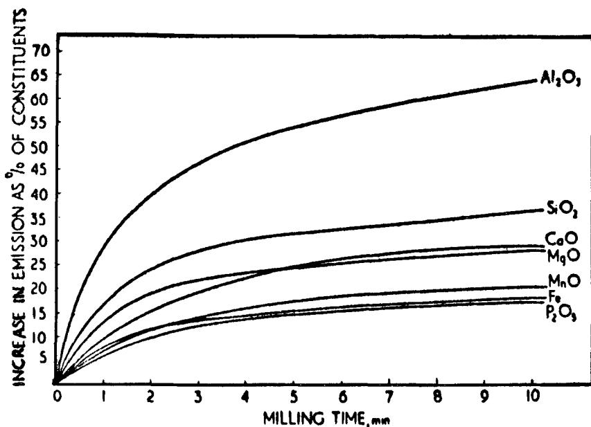
FIG. 1 -- Effect of particle size on emission.
