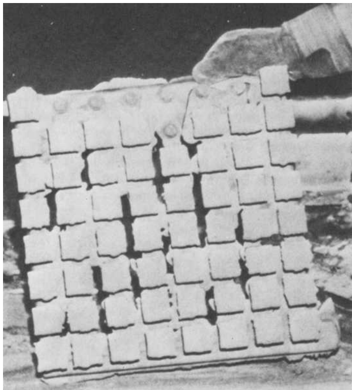
FIG. 2—Complete 64 sample block showing shrinkage tendency at extreme ends.
