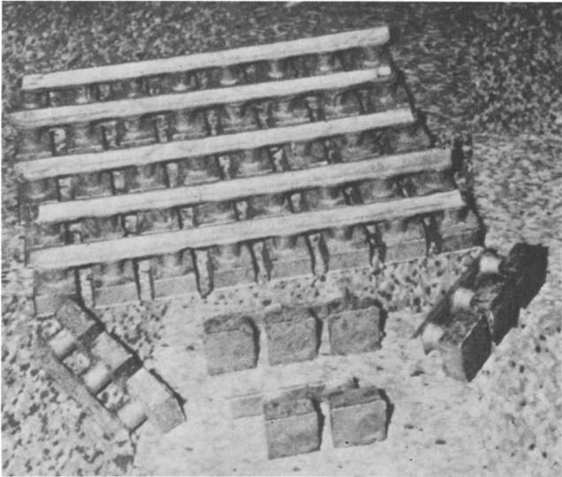
FIG. 6—Casting showing runners, ingates and samples.
