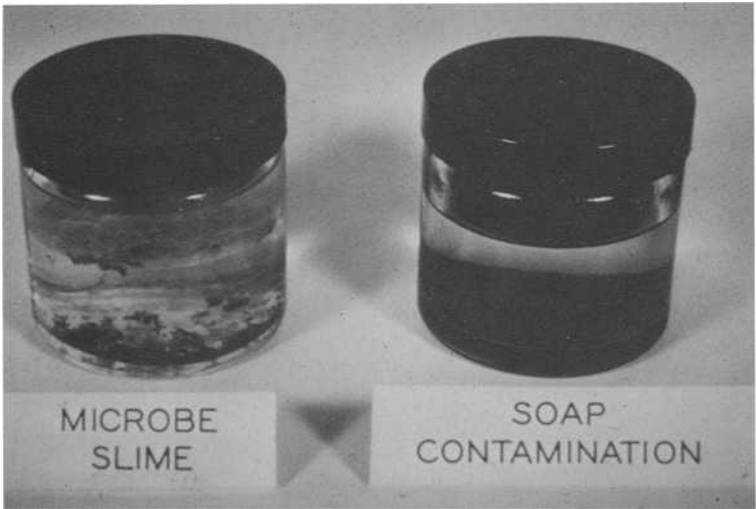
FIG. 11– Soap contamination and microbial slime.
