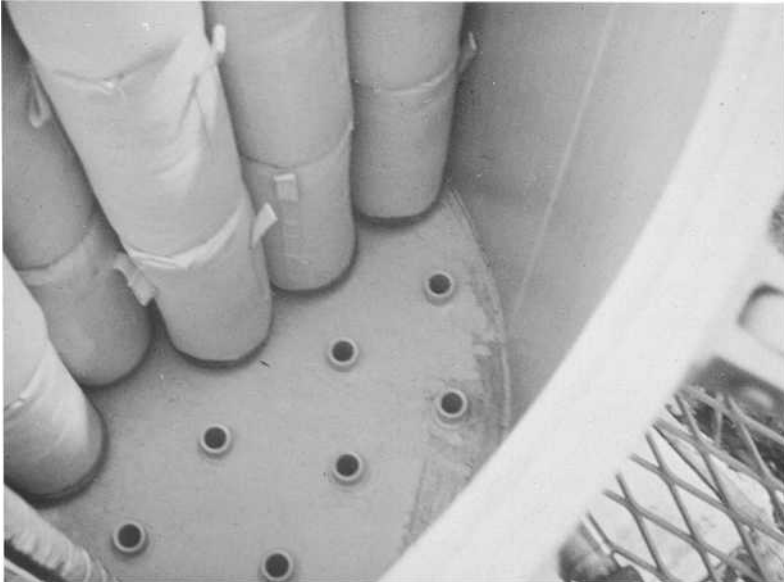
FIG. 13— Inside of a Fuller's earth filter (bag type).
