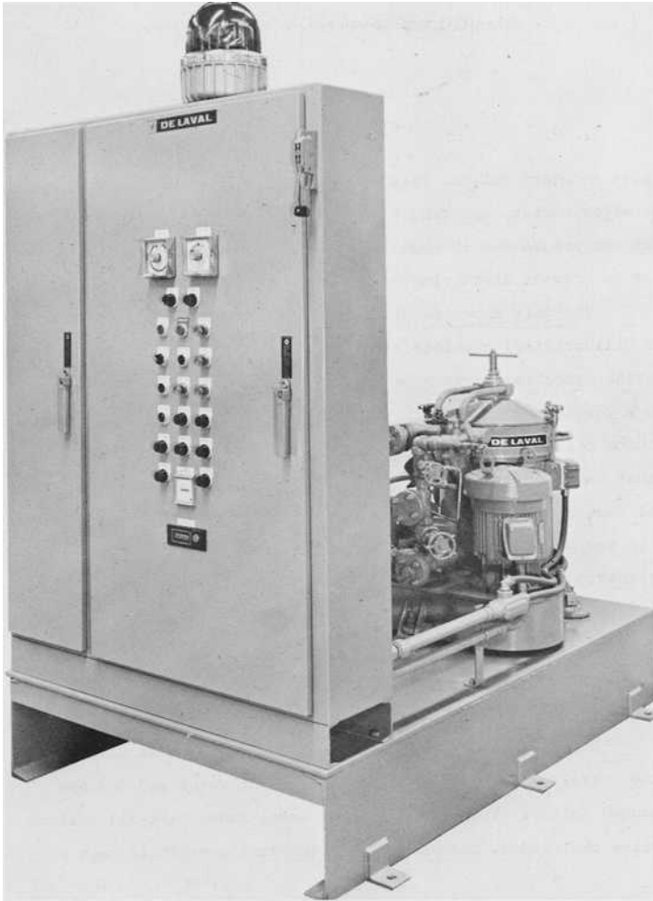
FIG. 4—Fuel oil purifier.
