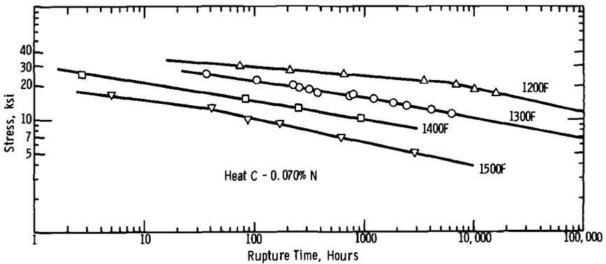
FIG. 4—Stress-rupture time properties of 0.07 percent nitrogen alloy.
