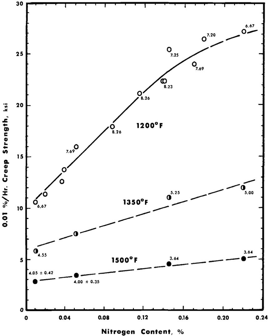
FIG. 3—Influence of nitrogen on the 0.01 percent per hour creep strength (based on minimum creep rate) of the nitrogen series heats at 1200, 1350, and 1500 F (649, 732, and 816 C). The numbers adjacent to the symbols are the stress exponent  $n$  for the relation  $\dot{\epsilon} = A\sigma^n$  at a minimum creep rate of 0.01 percent per hour. (To convert ksi to megapascals, multiply by 6.894757).
