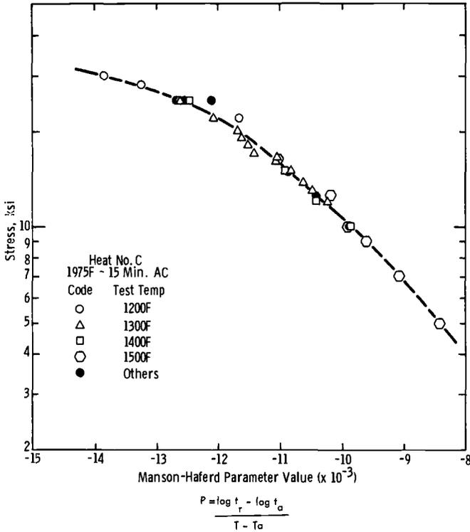
FIG. 19—Correlation of rupture data from 0.07 percent nitrogen alloy using Manson-Haferd parameter.
