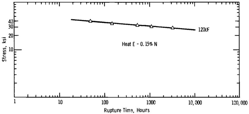
FIG. 6—Stress-rupture time properties of 0.15 percent nitrogen alloy.
