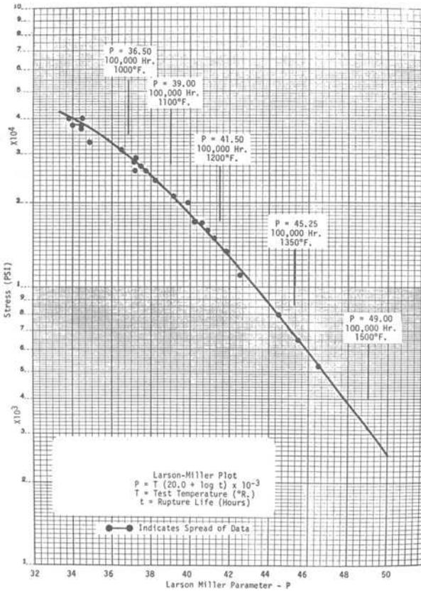
FIG. 7—Type 316N stainless steel stress-rupture tests data.
