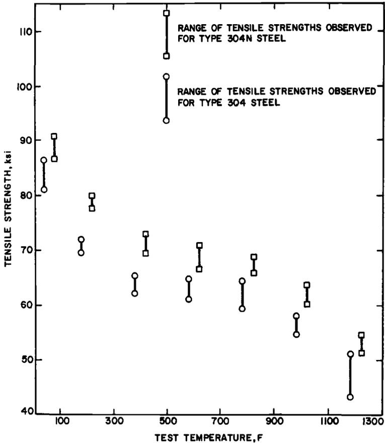
FIG. 5—Comparison of the room and elevated temperature tensile strengths of Types 304N and 304 stainless steels. (To convert from ksi to megapascals, multiply by 6.894757).
