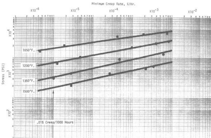
FIG. 8—Minimum-creep rate data, Type 304N stainless steel.
