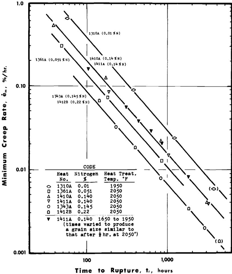
FIG. 5—Examples illustrating the type of relationship between minimum creep rate and time to rupture of tests of the nitrogen series heats at 1200 F (649 C).
