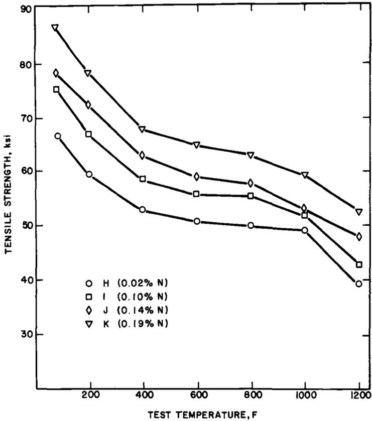
FIG. 7—Effect of test temperature on the tensile strength of Type 316L stainless steel containing nitrogen. (To convert ksi to megapascals, multiply by 6.894757).
