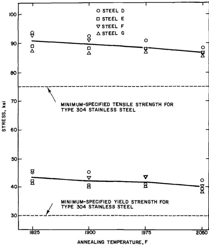
FIG. 3—Effect of annealing temperature on the room temperature yield and tensile strengths of Type 304N stainless steel. (To convert from ksi to megapascals, multiply by 6.894757).
