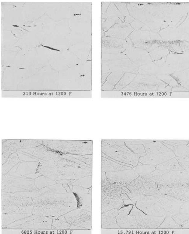
FIG. 11—Microstructures of ruptured specimens from Heat C (0.07 percent nitrogen). Etched in 10 percent oxalic acid ( $\times 500$ ).
