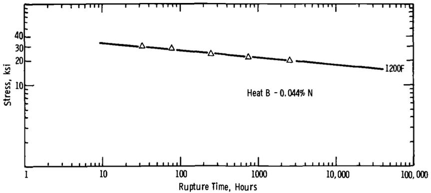
FIG. 3—Stress-rupture time properties of 0.044 percent nitrogen alloy.
