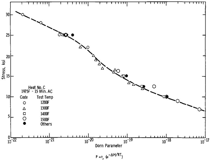
FIG. 17—Correlation of rupture data from 0.07 percent nitrogen alloy using Dorn parameter.
