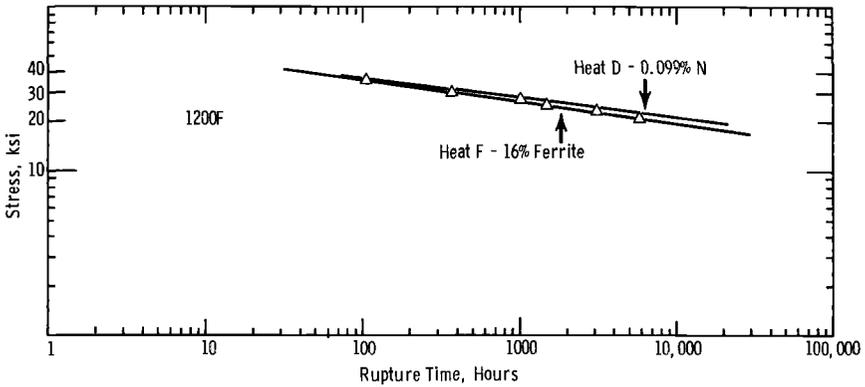
FIG. 13—Stress-rupture time properties of ferrite containing material compared to those of 0.099 percent nitrogen alloy.
