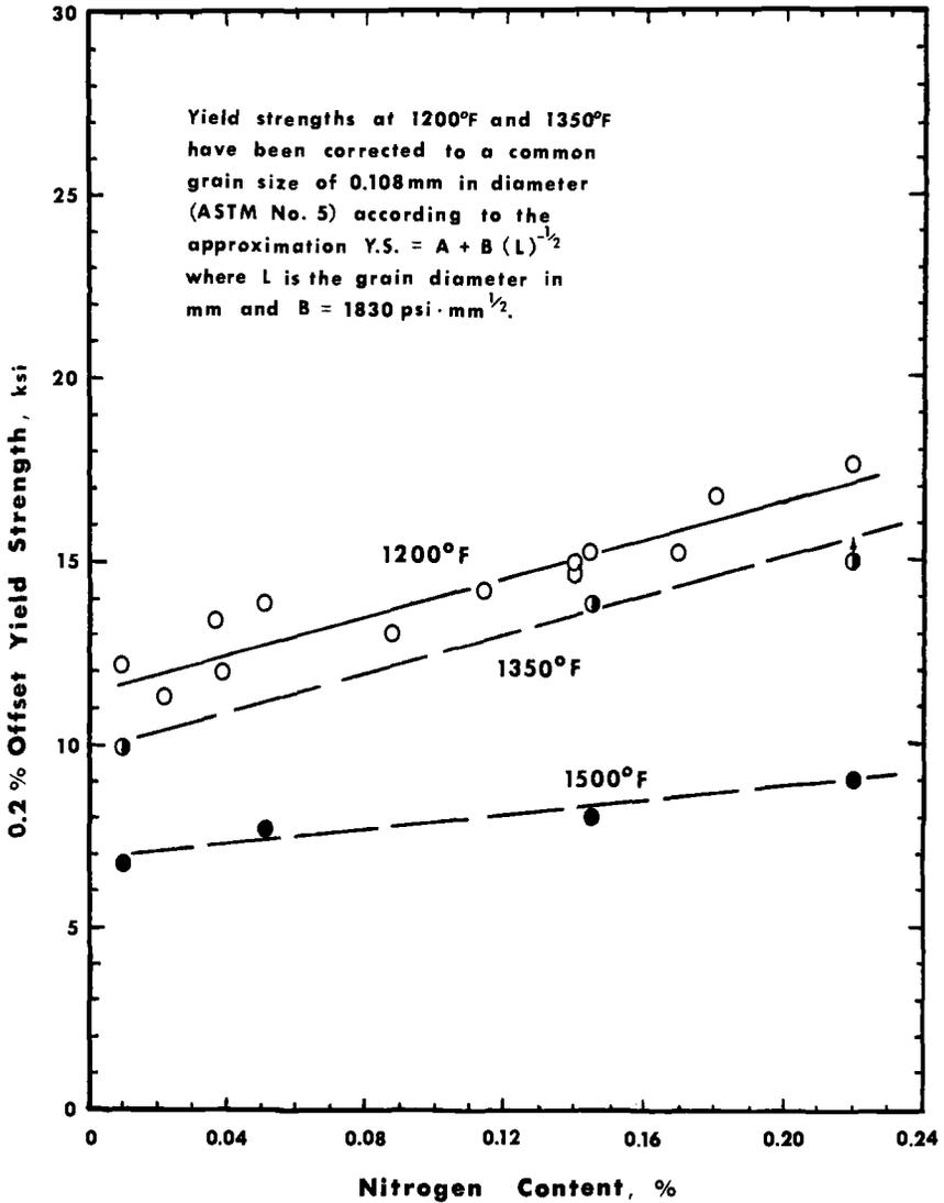
FIG. 2—Influence of nitrogen on the 0.2 percent offset yield strength of the nitrogen series heats at 1200, 1350, and 1500 F (649, 732, and 816 C). (To convert ksi to megapascals, multiply by 6.894757).
