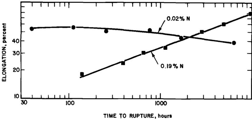
FIG. 8—Creep-rupture elongation at 1300 F (704 C) for Type 316L stainless steel containing 0.02 and 0.19 percent nitrogen.
