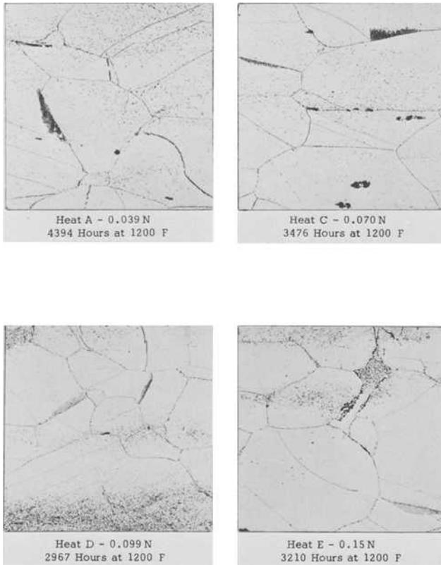
FIG. 12—Microstructures of specimens with different nitrogen contents having approximately equivalent rupture times at 1200 F (649 C). Etched in 10 percent oxalic acid ( $\times 1000$ ).
