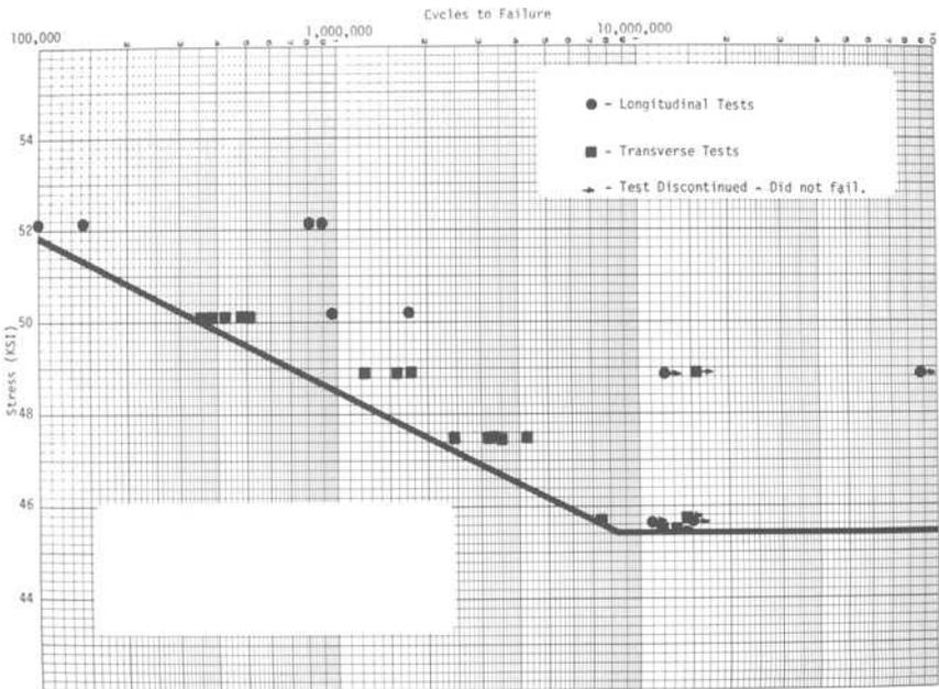
FIG. 10—Fatigue data, Type 304N stainless steel.
