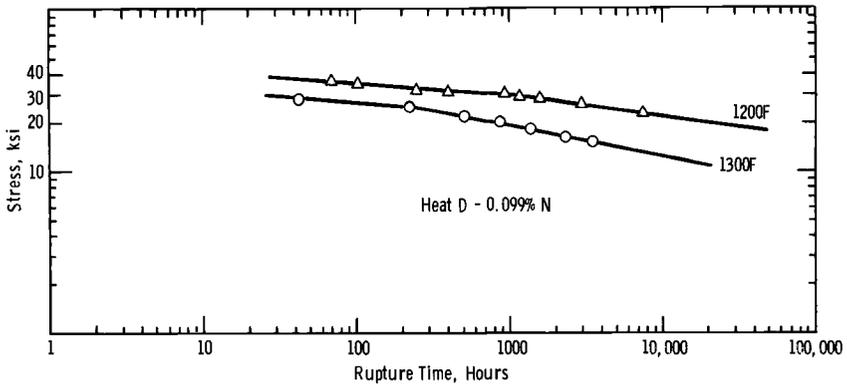
FIG. 5—Stress-rupture time properties of 0.099 percent nitrogen material.
