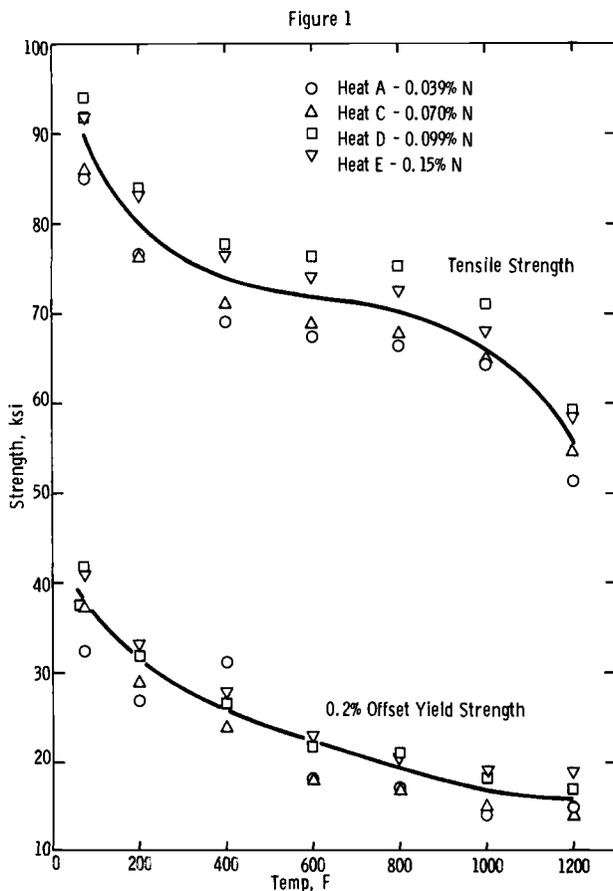
FIG. 1—Tensile and yield strengths of varying nitrogen alloys as a function of test temperature.
