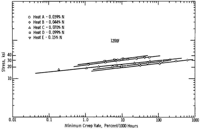
FIG. 9—Comparison of minimum-creep behavior at 1200 F (649 C) of varying nitrogen alloys.
