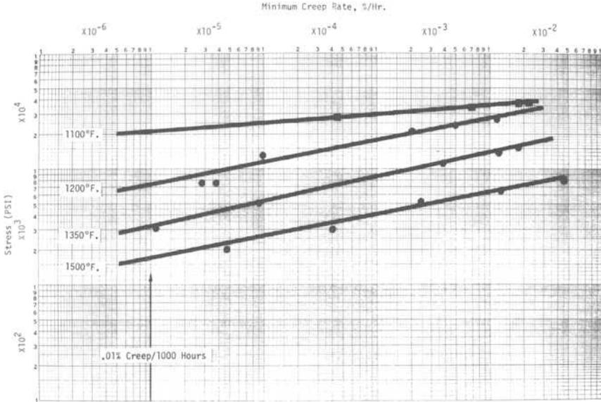
FIG. 9—Minimum-creep rate data, Type 316N stainless steel.
