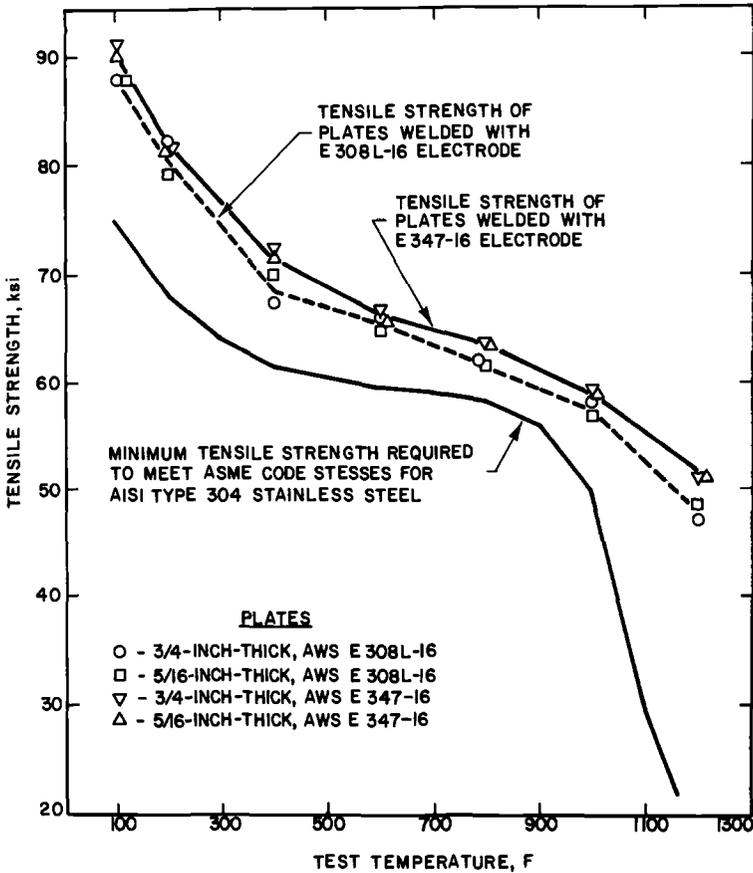
FIG. 2—Comparison of tensile strength of welded high-nitrogen Type 304L stainless steel plates with that required to meet ASME code stresses for AISI 304 stainless steel. (To convert ksi to megapascals, multiply by 6.894757).
