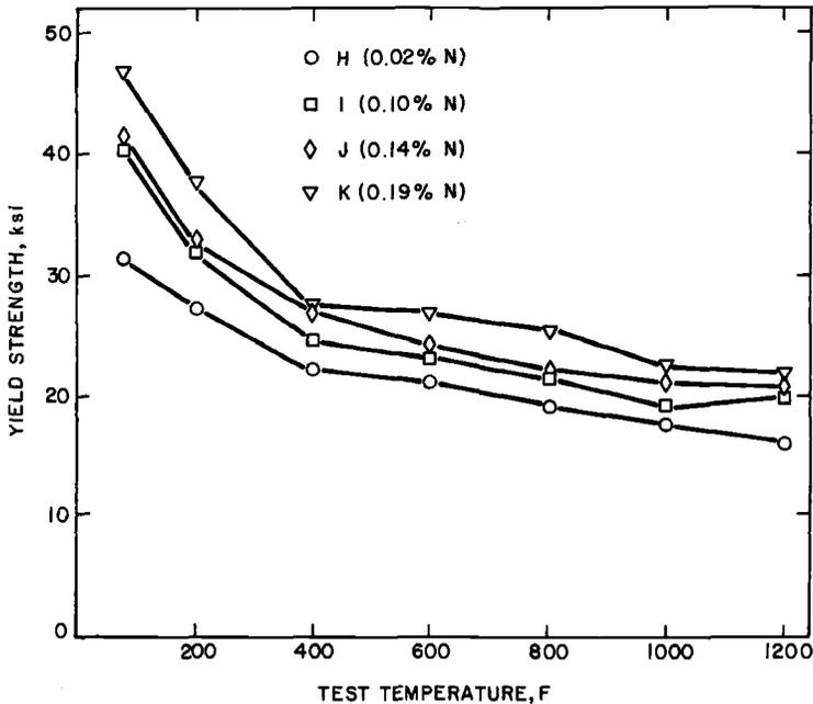
FIG. 6—Effect of test temperature on the yield strength of Type 316L stainless steel containing nitrogen. (To convert from ksi to megapascals, multiply by 6.894757).
