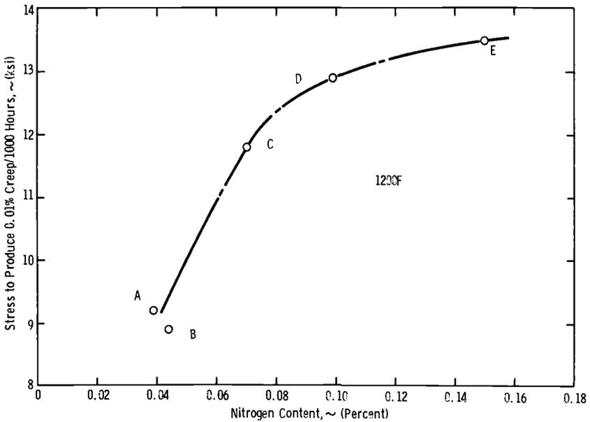
FIG. 10—Variation of stress to produce a minimum-creep rate of 0.01 percent per 1000 h with nitrogen content.
