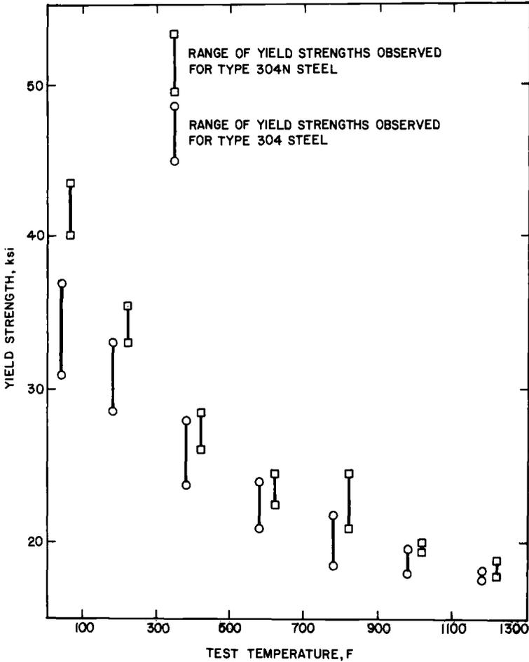
FIG. 4—Comparison of the room and elevated temperature yield strengths of Types 304N and Type 304 stainless steels. (To convert from ksi to megapascals, multiply by 6.894757).
