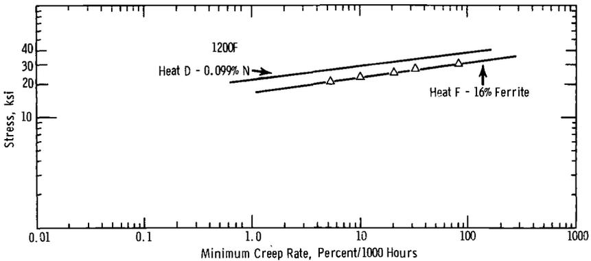
FIG. 14—Minimum-creep rate behavior of ferrite containing material compared to that of 0.99 percent nitrogen alloy.
