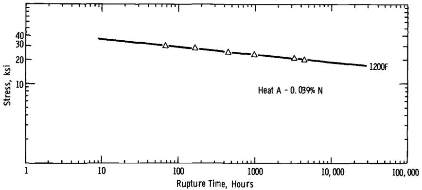
FIG. 2—Stress-rupture time behavior of 0.039 percent nitrogen material.
