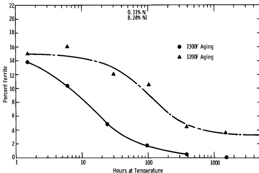
FIG. 15—Ferrite content of Heat F as a function of aging time.
