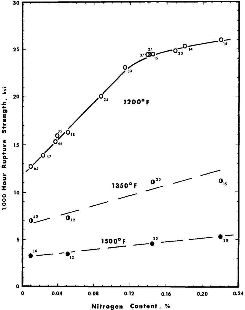
FIG. 4—Influence of nitrogen on the 1000-h rupture strength of the nitrogen series heats at 1200, 1350, and 1500 F (649, 732, and 816 C). The numbers adjacent to the symbols are the estimated elongation for rupture in 1000 h. (To convert ksi to megapascals, multiply by 6.894757).
