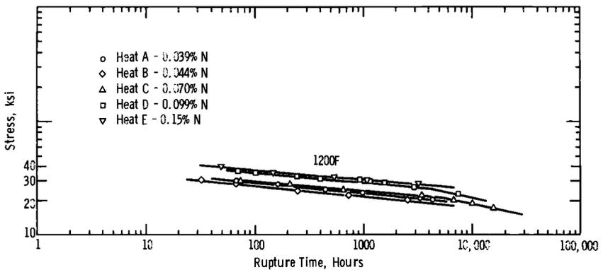
FIG. 7—Comparison of 1200 F (649 C) rupture properties of varying nitrogen alloys.
