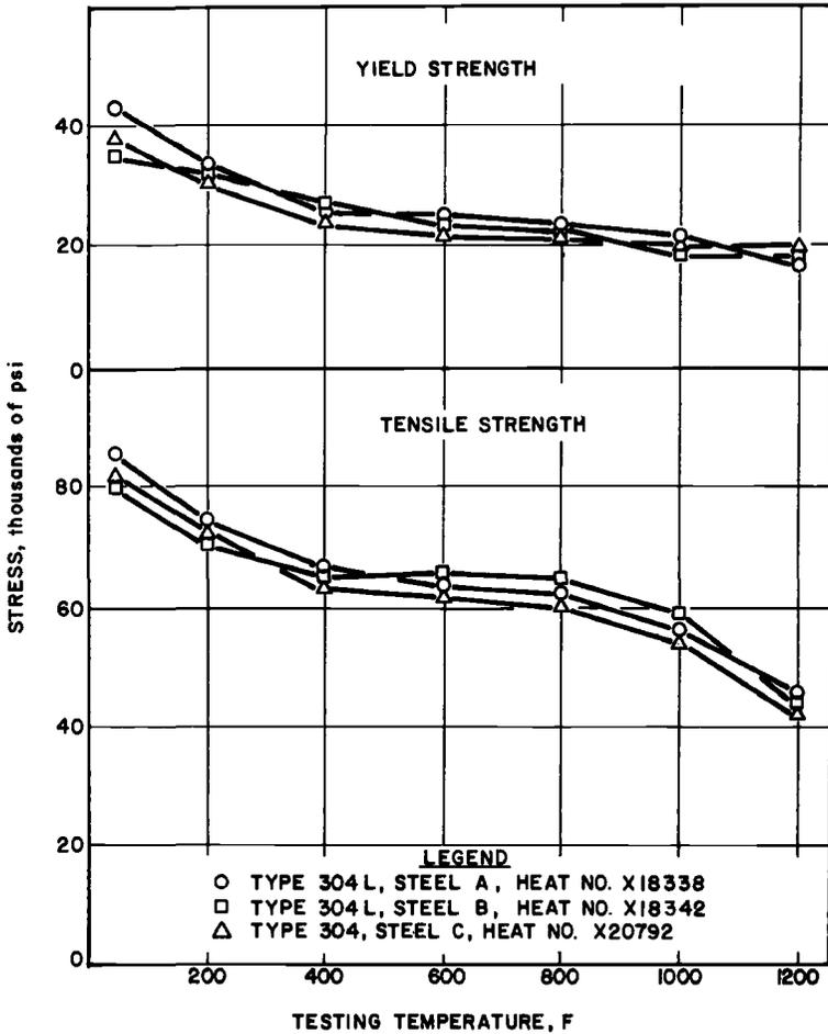
FIG. 1—Effect of temperature on the yield and tensile strengths of annealed high-nitrogen Type 304L and regular Type 304 steels. (To convert ksi to megapascals, multiply by 6.894757).
