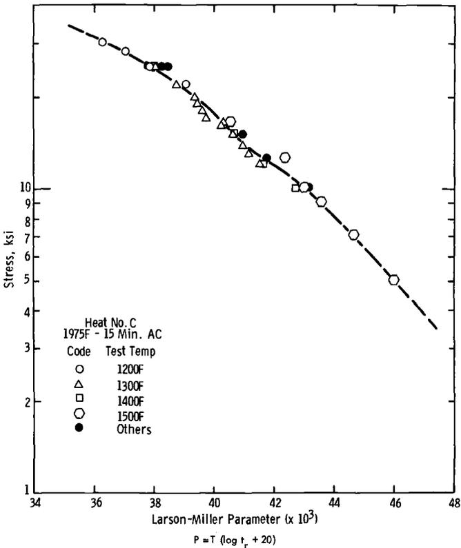
FIG. 18—Correlation of rupture data from 0.07 percent nitrogen alloy using Larson-Miller parameter.
