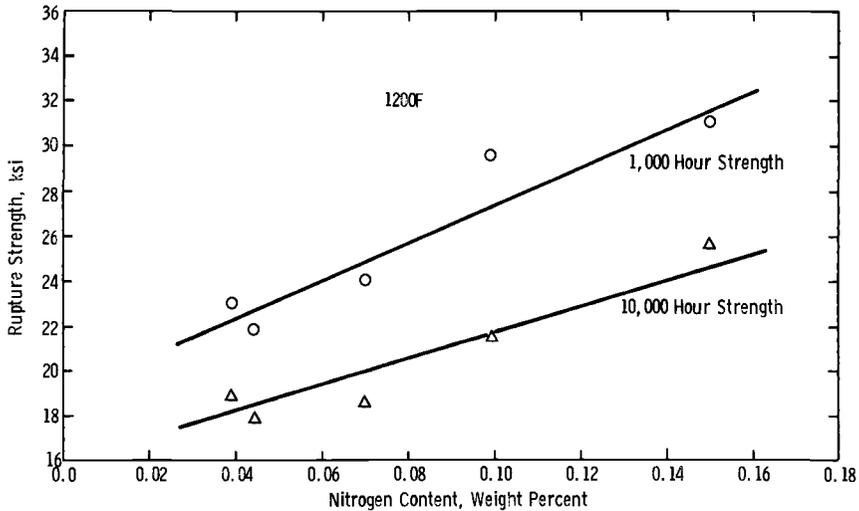
FIG. 8—Variation of 1000 and 10 000 h rupture strength at 1200 F (649 C) with nitrogen content.
