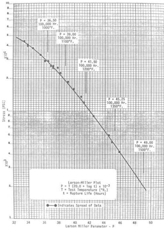
FIG. 6—Type 304N stainless steel stress-rupture test data.
