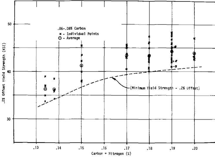
FIG. 1—Effect of carbon and nitrogen on Type 316 stainless steel yield strength.
