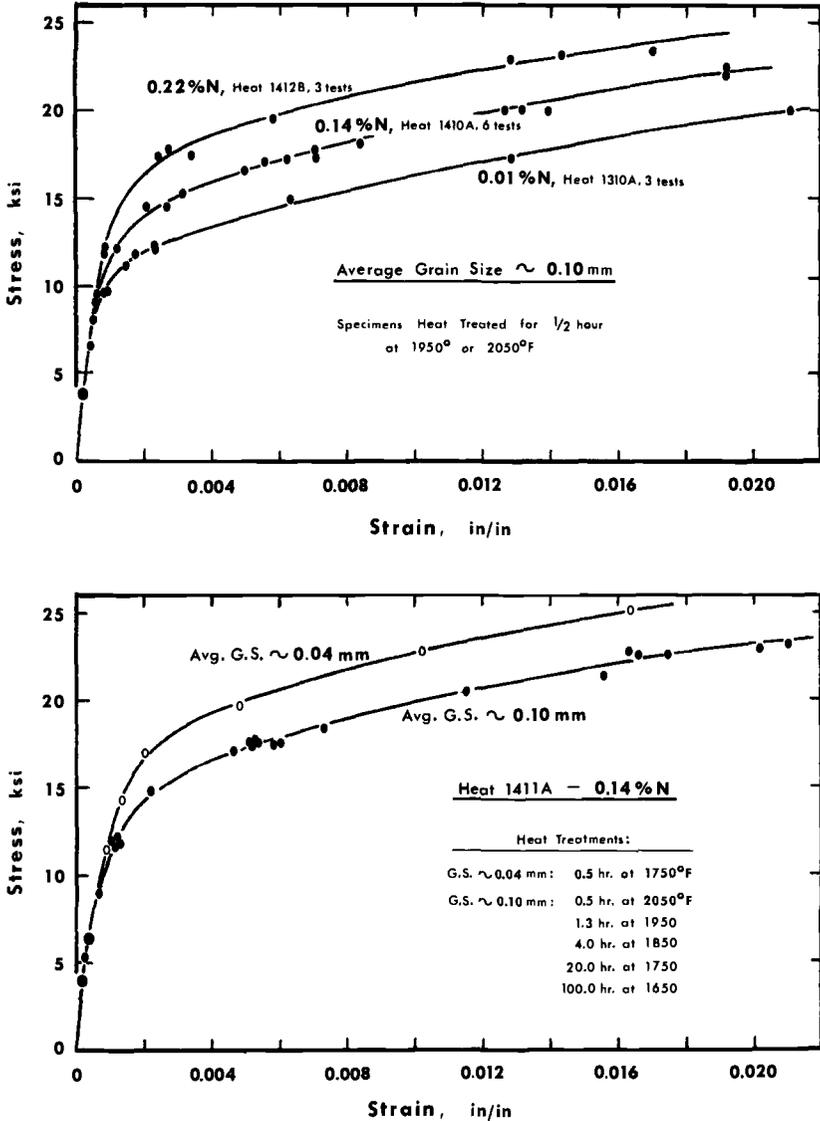
FIG. 1—Influence of nitrogen content and grain size on the 1200 F (649 C) stress-strain characteristics of several heats. These data are taken from loading of the creep-rupture tests. (To convert ksi to megapascals, multiply by 6.894757).
