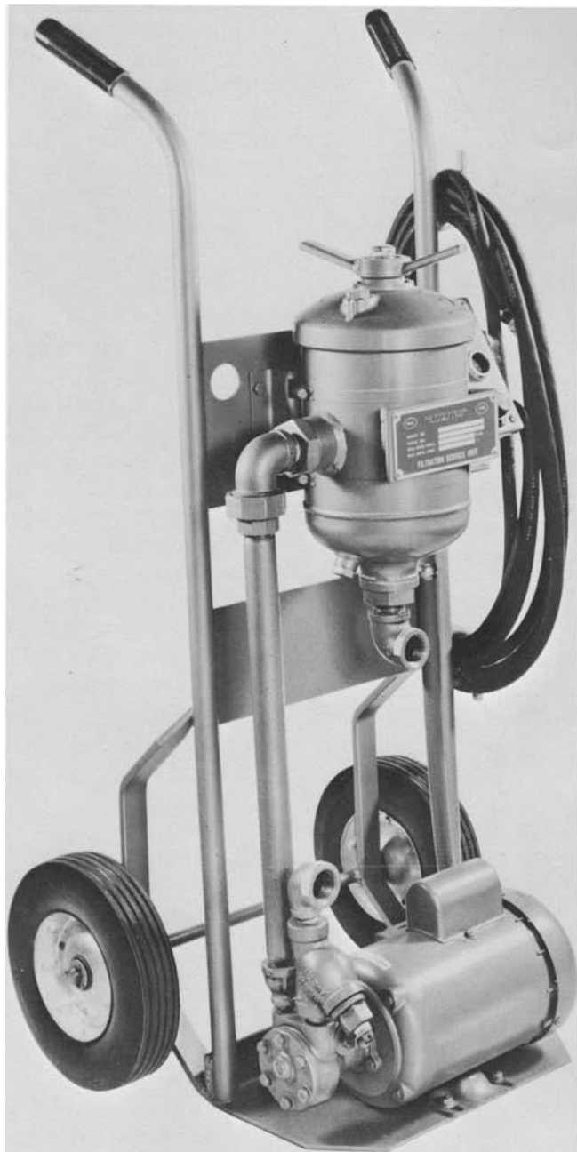
FIG. 10—A portable filtration unit.
