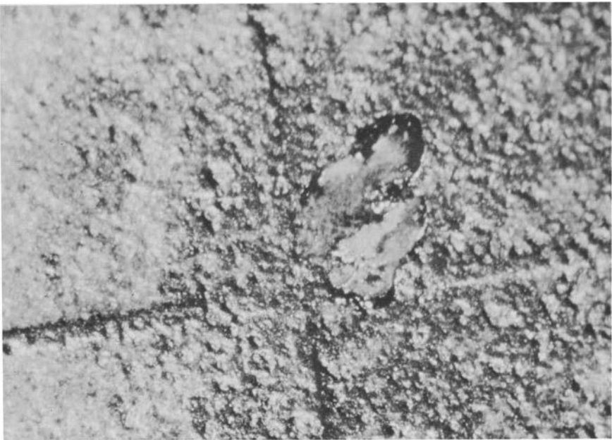
FIG. 4b—10W-30 oil with 1 percent water. Photographed at \times 8 magnification using bright field light. Analysis membrane shows a slimy deposit.
