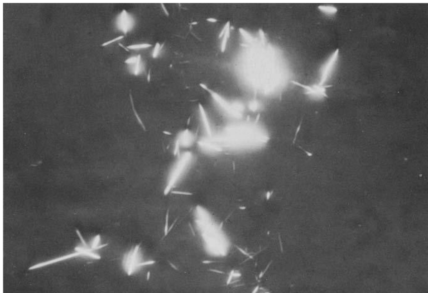
FIG. 5a—10W-30 oil with 1 percent water. Photographed at \times 200 magnification using polarized light, slightly uncrossed polars (85 deg). Needles approximately 30 to 40 \mu\text{m} long.
