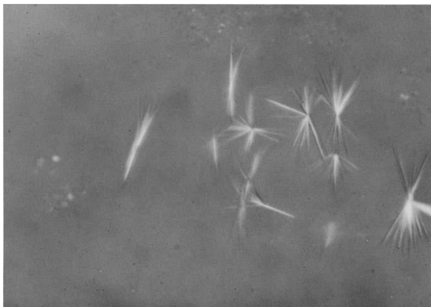
FIG. 5b—30 oil with 1 percent water. Photographed at \times 200 magnification using polarized light, slightly uncrossed polars (85 deg). Crystals approximately 50 \mu\text{m} .
