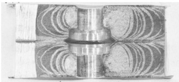
FIG. 19—Wing outer panel lower skin fatigue crack in bolt hole to diagonal spar.
