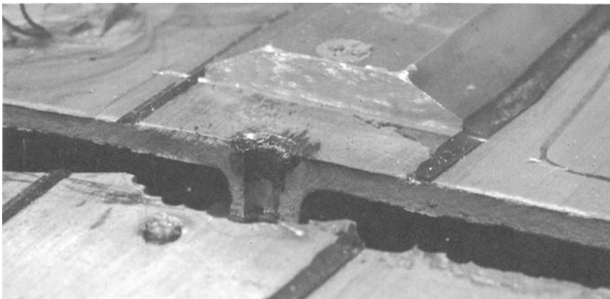
FIG. 17—Fatigue crack in lower skin wing outer panel 51 percent spar bolt hole with strap.
