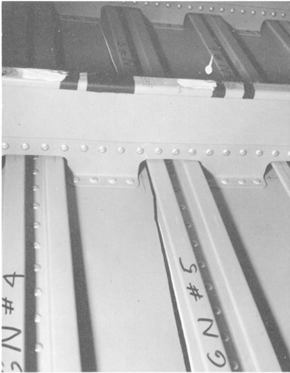
FIG. 20—Arrest of two-bay longitudinal crack after fast fracture, test 2, panel 3.
