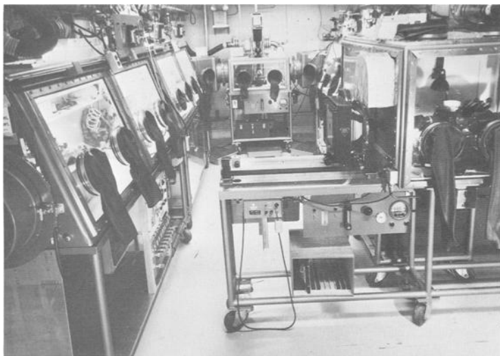
FIG. 2—Alpha metallography facility. Specimens which are high alpha radiation emitters must be prepared here.
