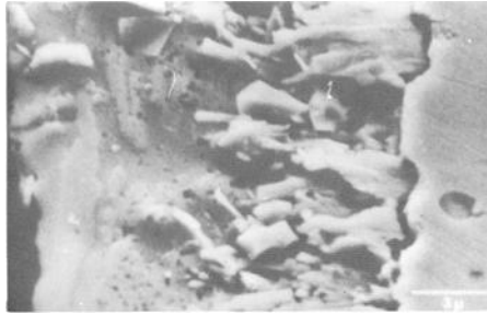
FIG. 25—Deeply etched cross section through zinc coating on sheet steel, showing crystal-line structure of intermetallic compound.
