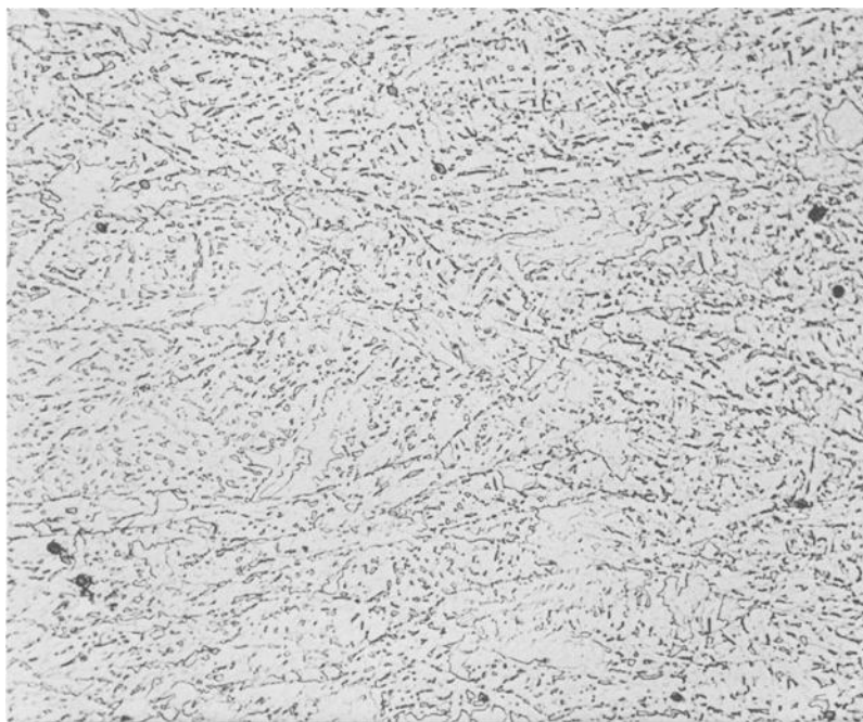
FIG. 7—Microstructure of Mo-B steel austenitized at 1040 C (1904 F), deformed to 50 percent reduction at 830 C (1526 F) and cooled at 300 C/min ( \times 460 ).
