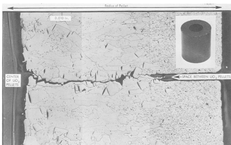
FIG. 18—Longitudinal view of two UO 2 pellets after irradiation. Inset shows typical UO 2 fuel pellet prior to irradiation.
