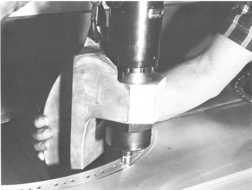
FIG. 18—Portable, hydraulic stress coin tool.
