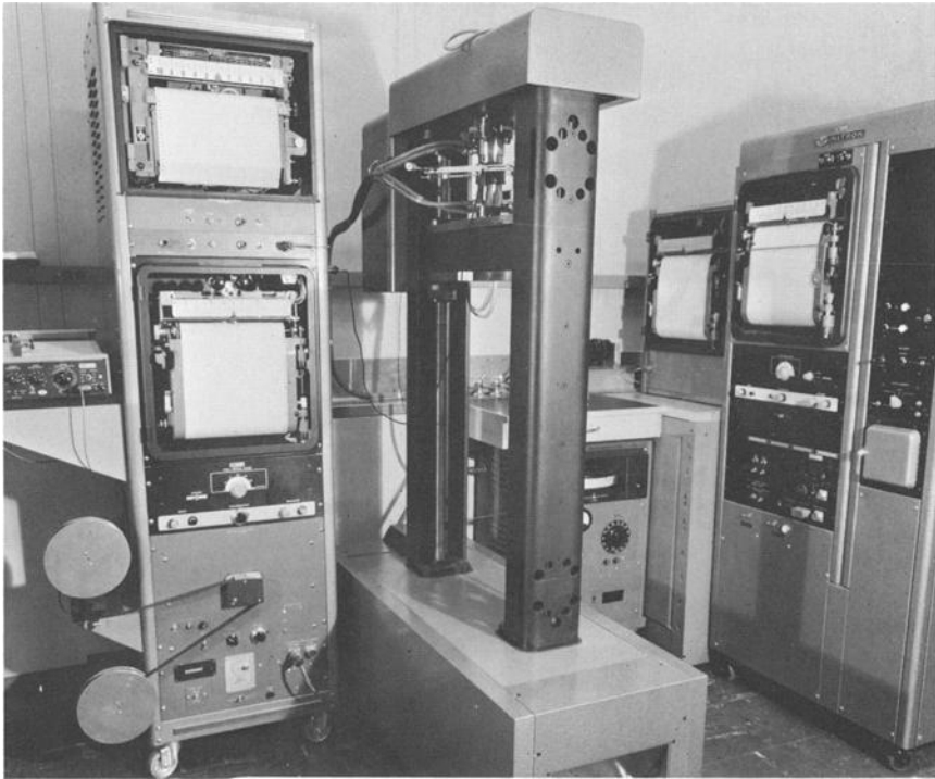
FIG. 2—Testing facility, including cyclic-monotonic strain programmer.
