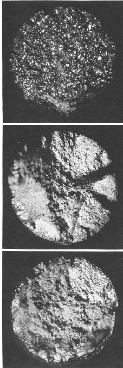
(left) Specimen A8: not heated intermittently; 145-ksi stress range; fatigue life = 189. (center) Specimen A11: not heated intermittently; 98-ksi stress range; fatigue life = 3100. (right) Specimen C1: heated 1400 times; 153-ksi stress range; fatigue life = 1750.
