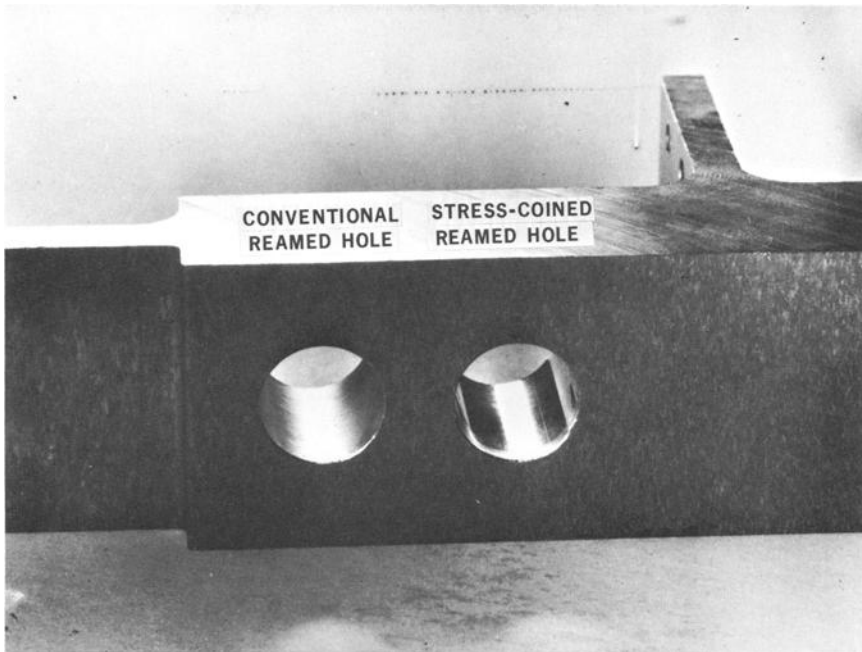
FIG. 4—Visual comparison of conventional and stress-coined holes.
