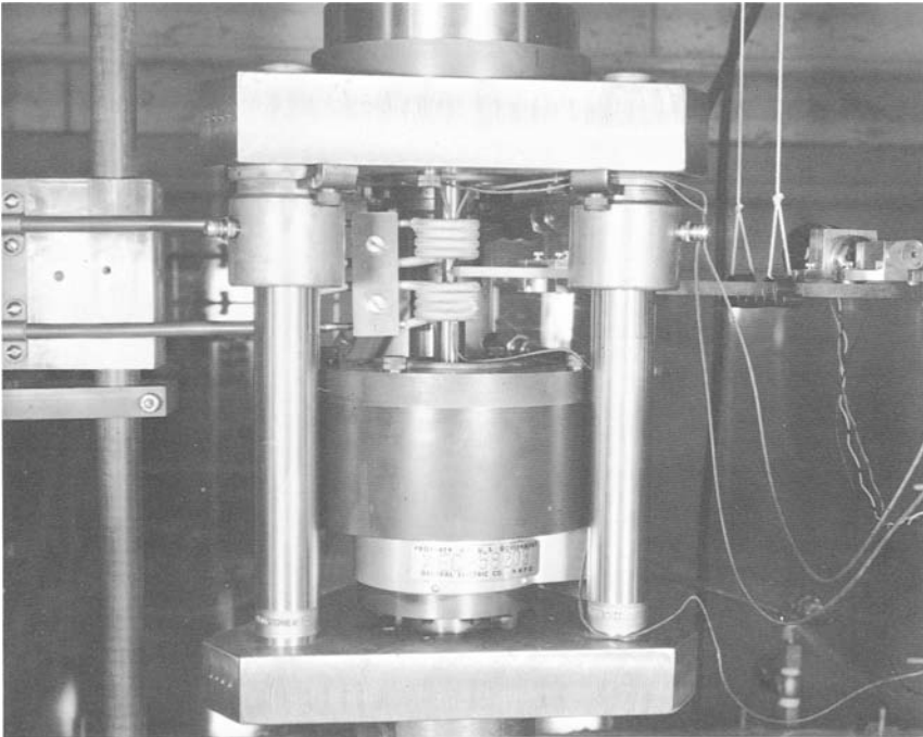
FIG. 4—Close-up view of loading fixture and induction coil.
