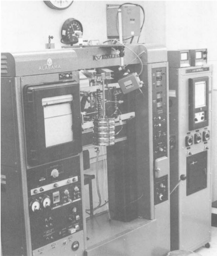
FIG. 4—Thermal fatigue test facility. Load cell calibration weights are visible.
