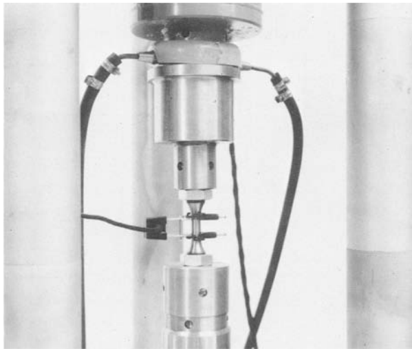
FIG. 14—Extensometer in mounted position.
