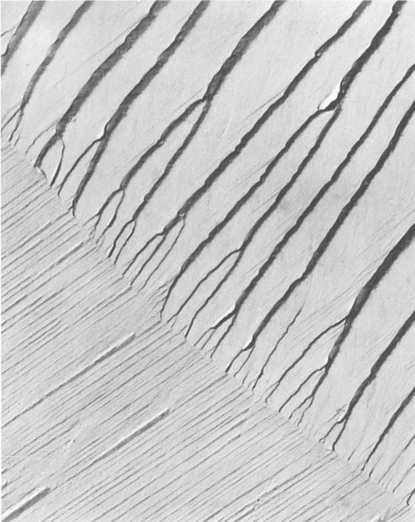
FIG. 8—River patterns on cleavage surface of ordered Fe-49Co-2V. After Johnston *et al* [14]. ( $\times 30,000$ ).
