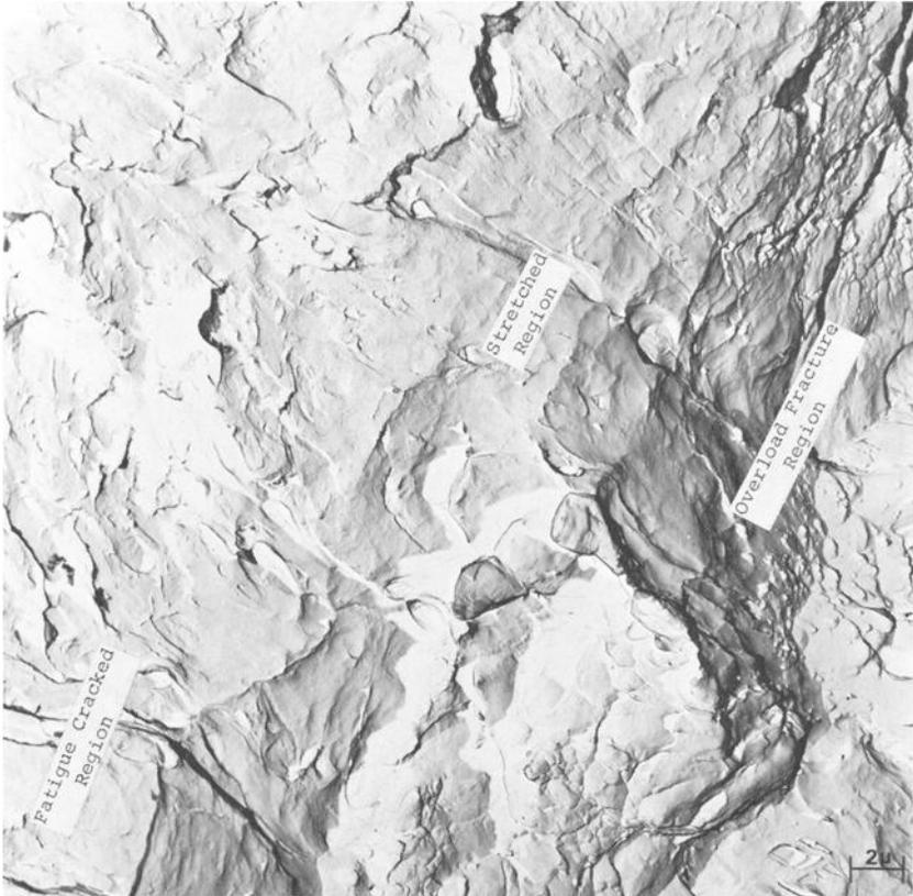
FIG. 8—Fracture surface of 250-grade maraging steel showing area between fatigue crack and overload fracture regions.
