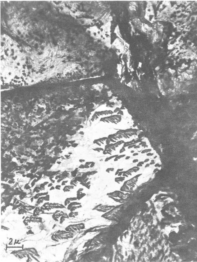
FIG. 18—Fracture of irradiated fuel cladding (Type 304 steel) at 600 C superheat. Extraction replica [32] ( $\times 3750$ ).
