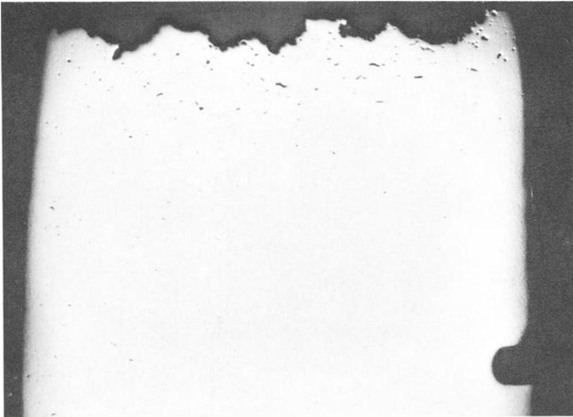
FIG. 11—Intergranular microcracks formed during creep of a CrMoV low-alloy steel at 1050 F stressed for 7700 h at 25,000 psi ( $\times 10$ ).
