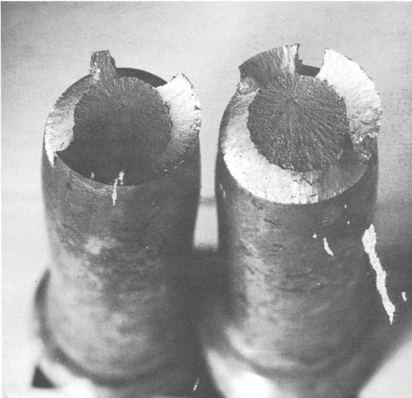
FIG. 14—Macroscopic view of AISI 4340 cup-and-cone fracture surface from which the fractograph in Fig. 13 was made. Fracture initiation region may be seen just above the center of the fracture surface ( $\times 4$ ).
