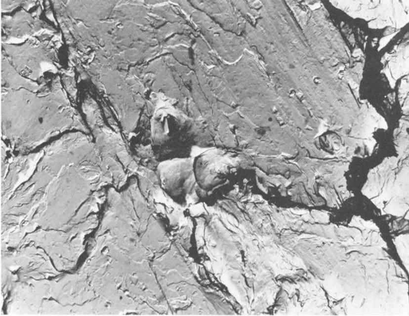
FIG. 13—Fracture surface topography of Type 304 smooth-bar tension specimen exposed 24 h and pulled to fracture in 10,000 psi hydrogen. After Vennett and Ansell [41]. Two-stage plastic-carbon replica ( $\times 5300$ ).
