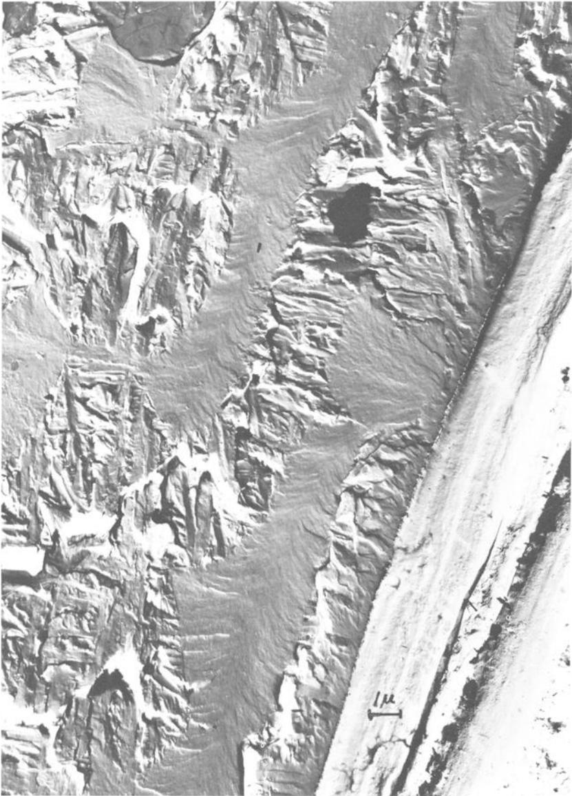
FIG. 11—SCC in Ti-6A-4V alloy exposed to methanol [21] (crack initiated at machining mark on right) ( $\times 6000$ ).
