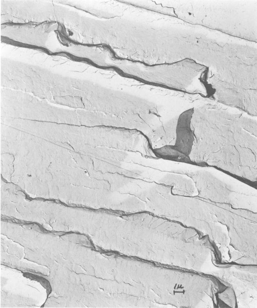
FIG. 12—SCC in Ti-7Al-2Cb-1Ta alloy exposed to distilled water [21] ( $\times 4000$ ).
