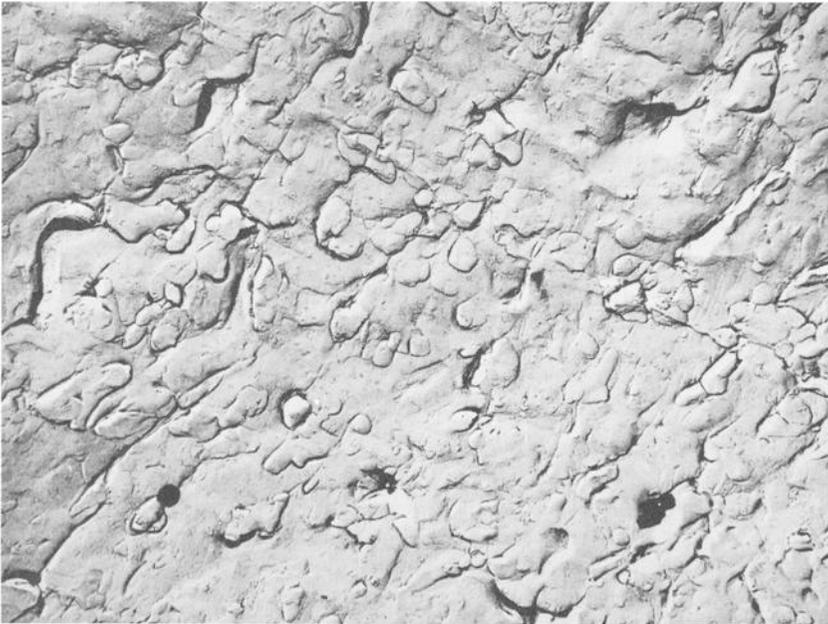
FIG. 13—Fractographic features of exposed microcrack surface showing distribution of particle sites ( $\times 5000$ ).
