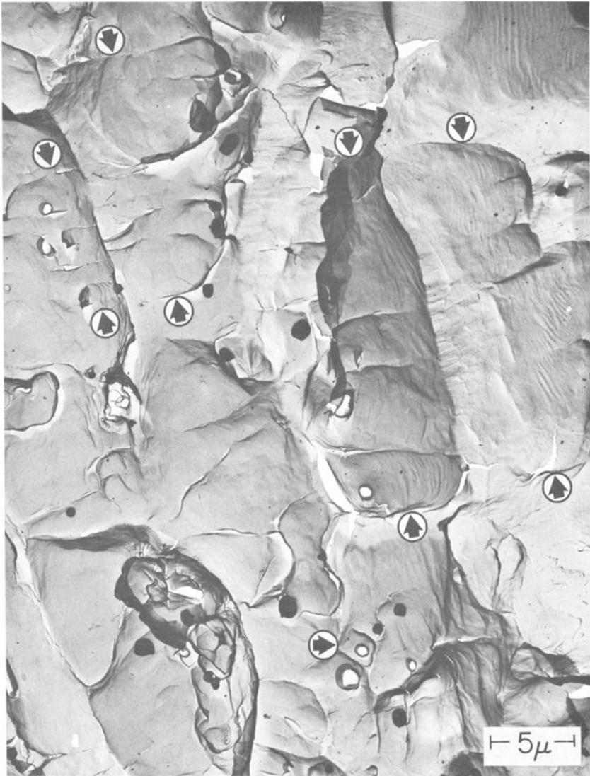
FIG. 12—Examples of serpentine glide in dimples in tough pitch copper. Specimen alligatored due to residual stresses from rolling. An equiaxed dimple is shown by the horizontal arrow. Tear dimples are shown between slanted arrows. Palladium-shadowed direct-carbon replica ( $\times 5000$ ).
