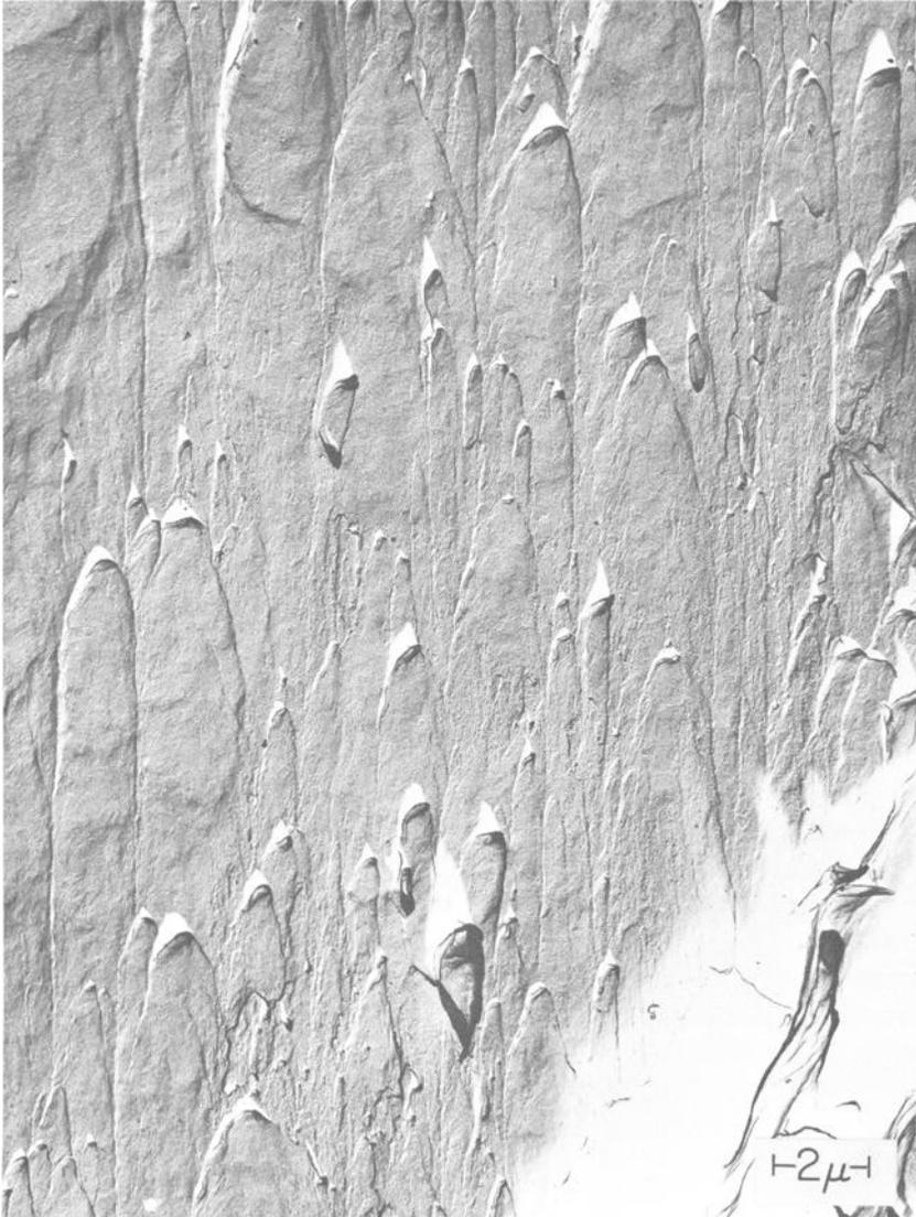
FIG. 25—Long shear rupture dimples in an OFHC copper torsion rupture surface. Two-stage palladium-shadowed carbon replica ( $\times 9000$ ).
