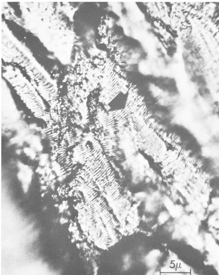
FIG. 1—*Optical fractograph of fatigue striations in an aluminum alloy.*
