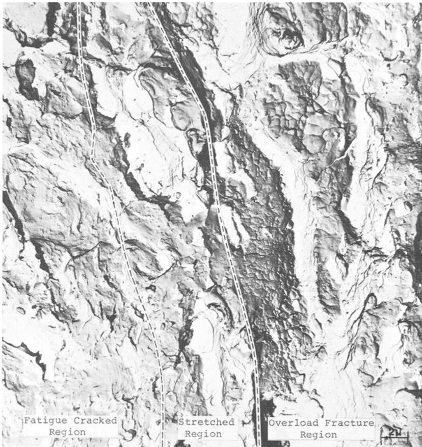
FIG. 5—Fracture surface of 0.45C-Ni-Cr-Mo steel with 0.008 per cent sulfur showing area between fatigue crack and overload fracture regions.
