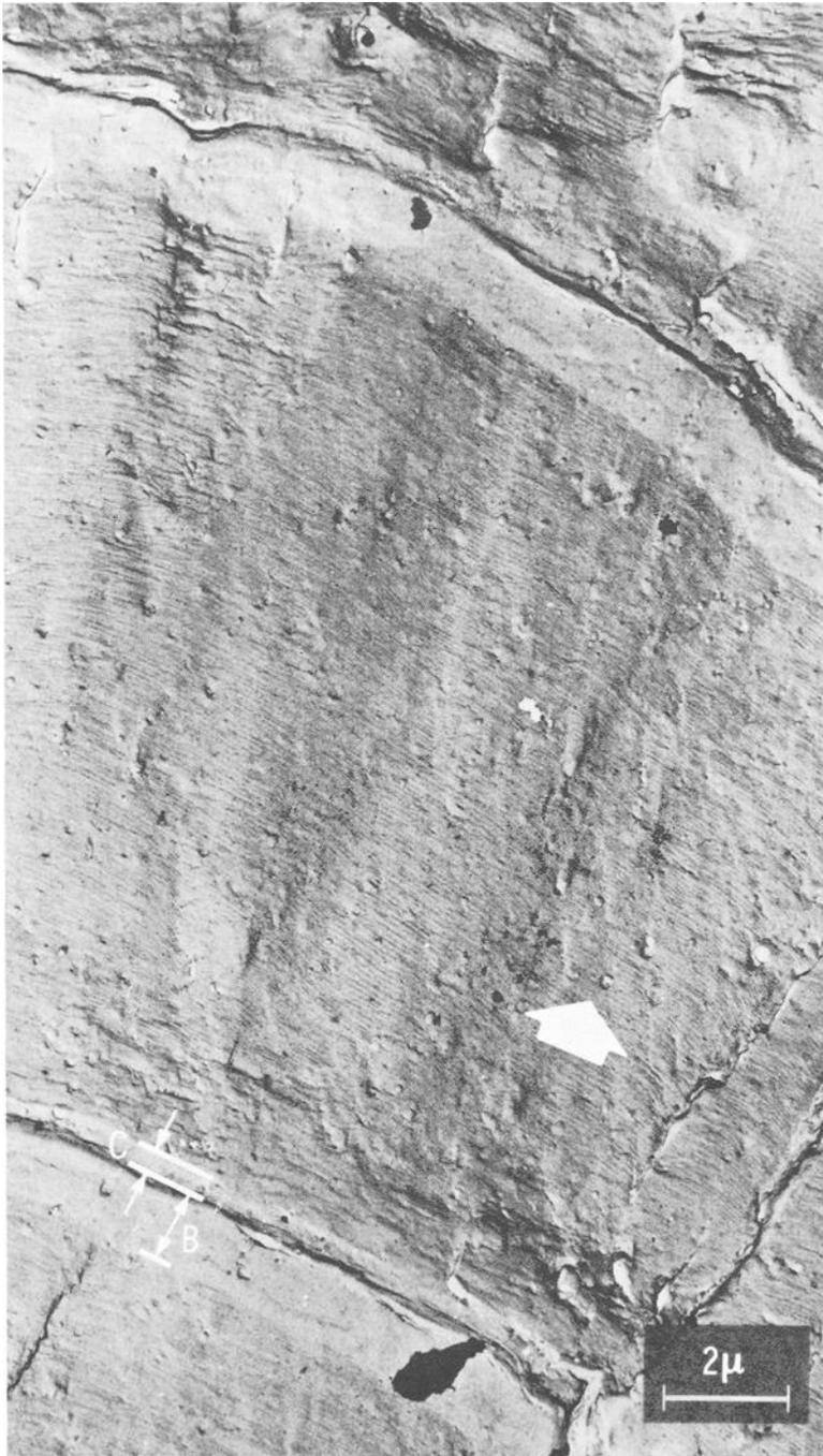
FIG. 9—Fracture topography resulting from application of program P 15.
