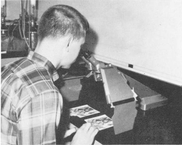
FIG. 5—Examination of stereo-pairs in a special viewer to observe the three-dimensional characteristics of a fracture.
