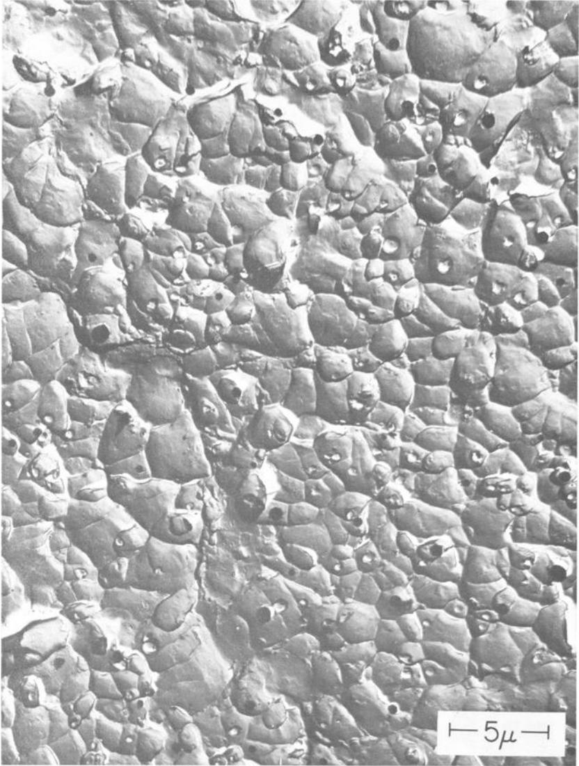
FIG. 17—Equiaxed dimples in a hardened-and-tempered low-alloy steel specimen. Palladium-shadowed two-stage carbon replica ( $\times 6000$ ).
