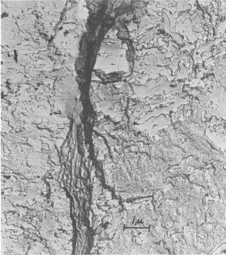
FIG. 2—Stress-corrosion fracture of Type 301 stainless steel in 10 per cent  $\text{FeCl}_3$ , room temperature ( $\times 11,600$ ).
