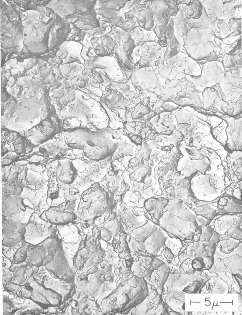
FIG. 16—Equiaxed dimples in the AMS 6434. Two-stage palladium-shadowed carbon replica ( $\times 6000$ ).
