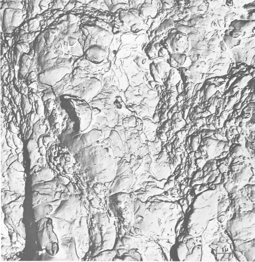
FIG. 3—Fracture surface of 0.45C-Ni-Cr-Mo steel with 0.008 per cent sulfur showing area adjacent to fatigue crack.
