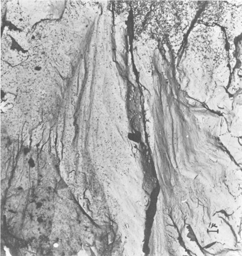
FIG. 7—Electron micrograph of “feather” area of Fig. 7 ( $\times 4000$ ).
