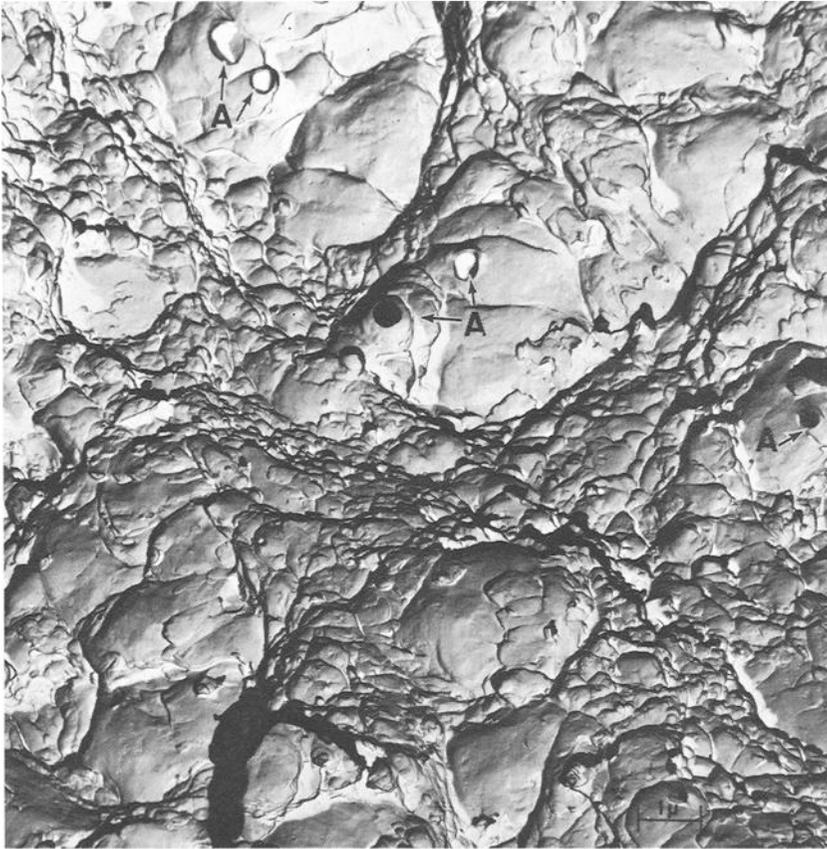
FIG. 4—Fracture surface of 0.45C-Ni-Cr-Mo steel with 0.049 per cent sulfur showing area adjacent to fatigue crack.
