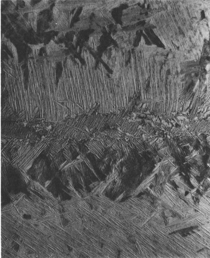
FIG. 17—*Typical microstructure of Ti-721 annealed at 1750 F.*
