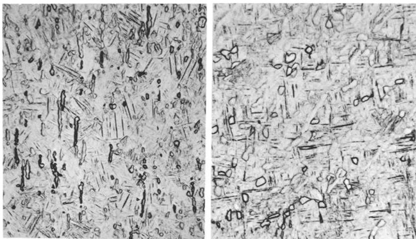
FIG. 1—Conventional solution treated, water quenched, and aged microstructures of (a) medium and (b) low interstitial heats of 6Al-4V titanium ( $\times 250$ ).
