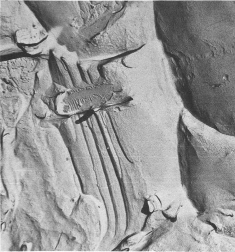
FIG. 8—*Electron fractograph of crack path through and around alpha platelet ( $\times 13,000$ ).*
