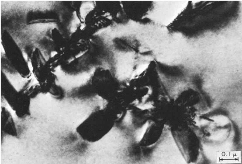
FIG. 11—Transmission electron micrograph of (900 F/8 hr) aged B-120VCA, showing alpha precipitates with Moiré fringe contrast.
