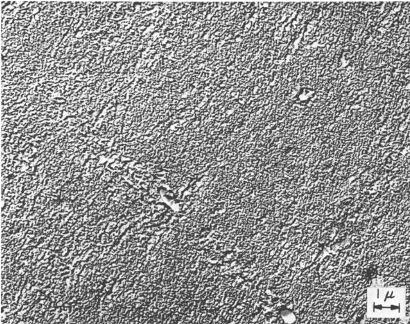
FIG. 14—Surface replica electron micrograph of 65 per cent cold-rolled and -aged (900 F/72 hr) specimen showing finely dispersed alpha precipitate.
