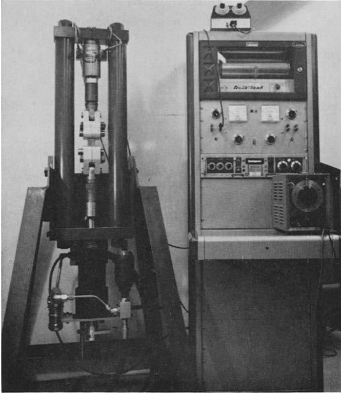
FIG. 58—Hydraulic tester used as an axial fatigue machine to grow short, deep cracks.
