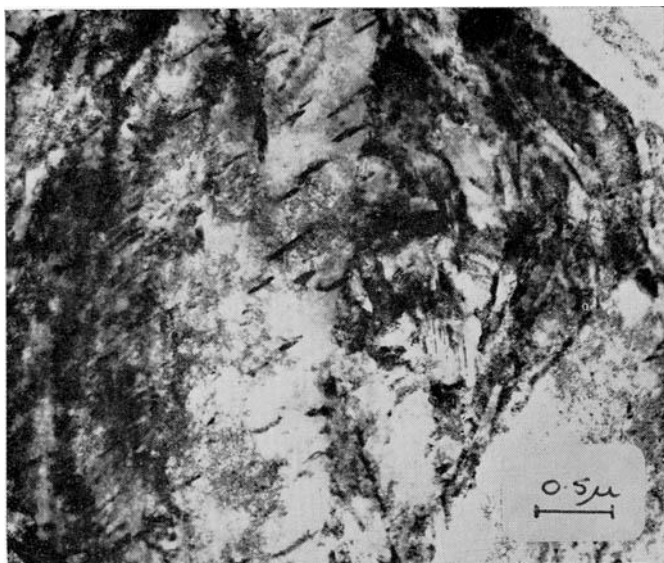
FIG. 7—En 30B (Cast B 7365). Ausformed and tempered at 400 C (750 F). Thin foil ( \times 20,000 ). Coarse cementite precipitation.
