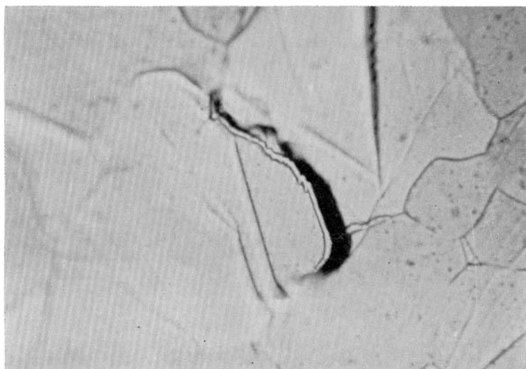
FIG. 15—Example of ferrite-cementite interface crack in Fe-0.02C-0.07Sb alloy embrittled for 24 h at 480 C and tested in tension at 77 K. Tensile axis horizontal ( \times 500 ) (Ref 44).
