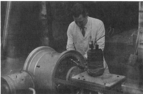
**Fig.6. MIL-H-5606 burning at 600C brake temperature.**
