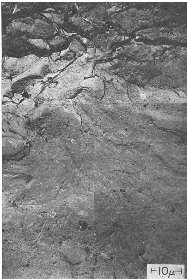
FIG. 38—Composite Electron Microscope Fractograph of One of the Cracks in Fig. 37 Showing Striated Fatigue Fracture Originating from a Minute Intergranular Surface Flaw. Two-Step Replica. 2400 \times . Reduced One Third in Reproduction.
