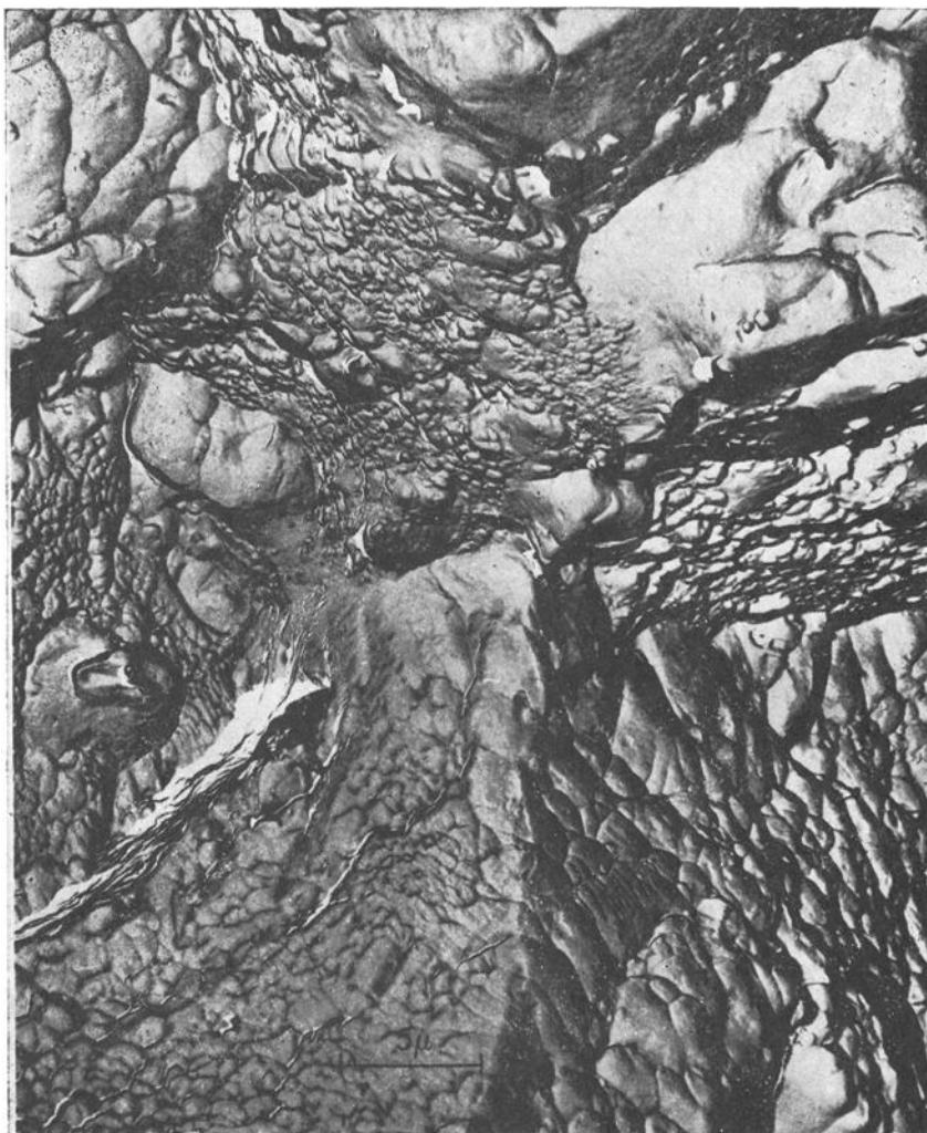
FIG. 20—Intergranular Fracture, due to Micro-void Coalescence, in a 2219 Alloy.
