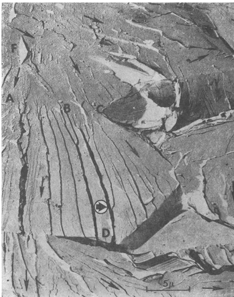
FIG. 2—Cleavage Fracture Surface of a Low-Carbon Steel Broken by Impact at 78 K.
