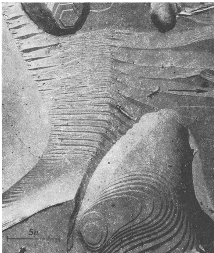
FIG. 22—Cleavage Fracture and Separation Along the Interface of a Large Particle in an Alnico Alloy.
