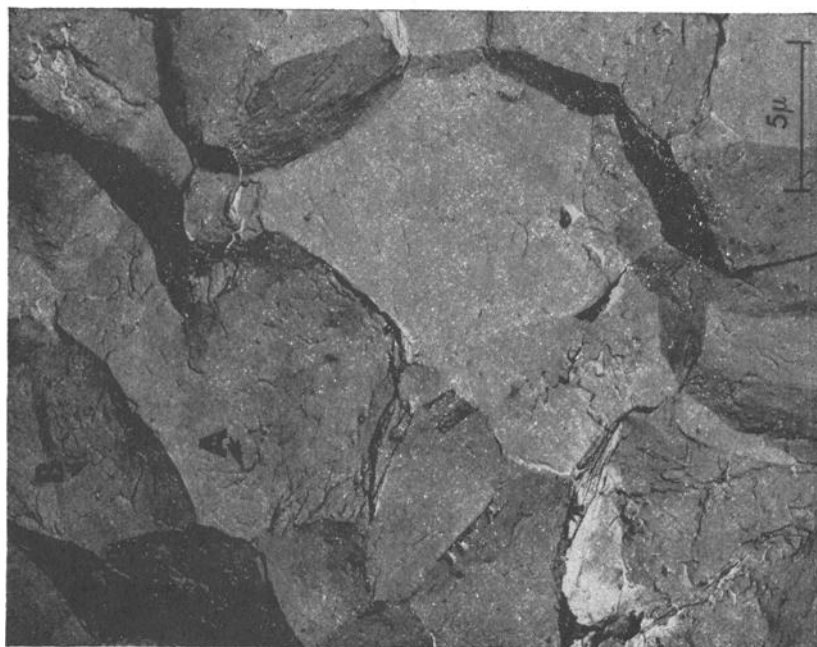
FIG. 25—Intergranular Fracture in a 4340 Steel. This intergranular fracture at the origin of a service failure was probably due to stress corrosion and hydrogen embrittlement. Note the tear ridges along the grain-boundary facets and the dimples in A and B. Two-step replica. (Reprinted from Ref (3).) 6000X. Reduced one third in reproduction.
