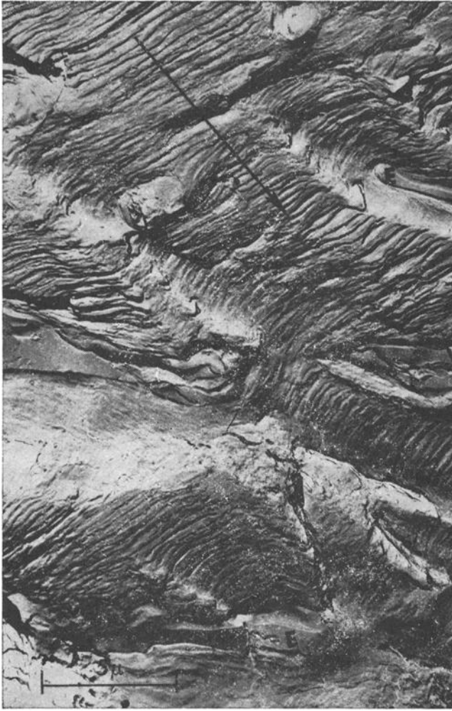
FIG. 34—Fatigue Striations in a Welded Zone of a 2219 Aluminum Alloy.
