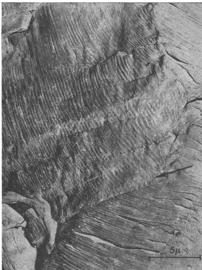
FIG. 35—Fatigue Striations in a Zirconium Alloy. Two-Stage Replica. 6400 \times . Reduced One Third in Reproduction.
