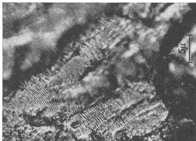
FIG. 26—Optical Micrograph of a Fatigue Fracture in a 7178 Aluminum Alloy. Some Regions Are out of Focus due to the Small Depth of Field of the Optical Microscope. 3200X. Reduced One Third in Reproduction.
