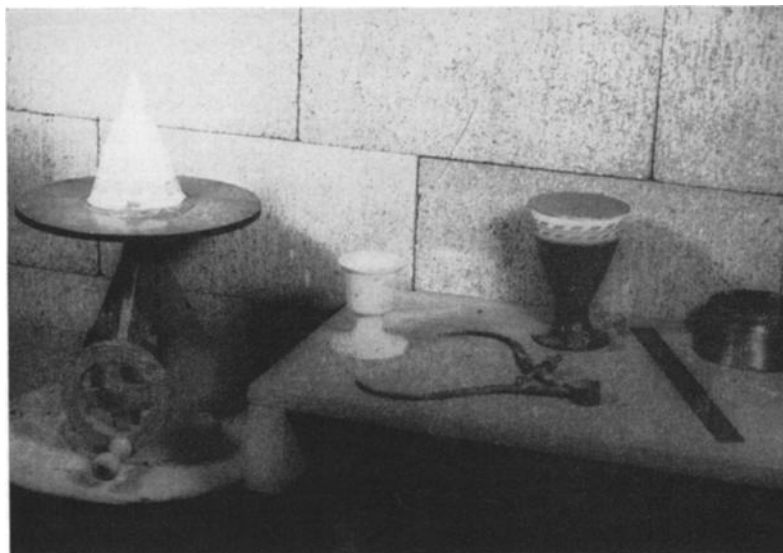
FIG. 6.—Material for Test for Consistency of Hydraulic Cement Showing the Paper Cones Used as Molds.
