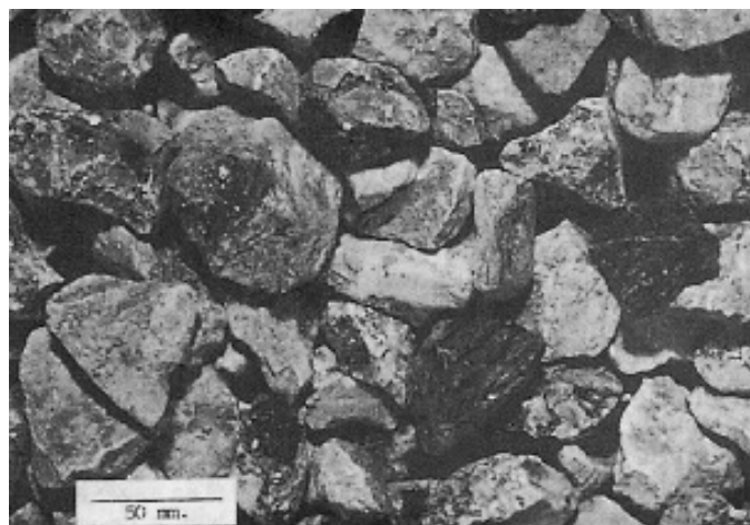
Fig. 9 —Crushed limestone aggregate containing seams and pieces of illite shale, Webster Dam, Kansas. The physical quality was indicated as follows: satisfactory, 61 %; fair, 34 %; poor, 5 % by mass (courtesy of the Bureau of Reclamation, U.S. Department of the Interior).
