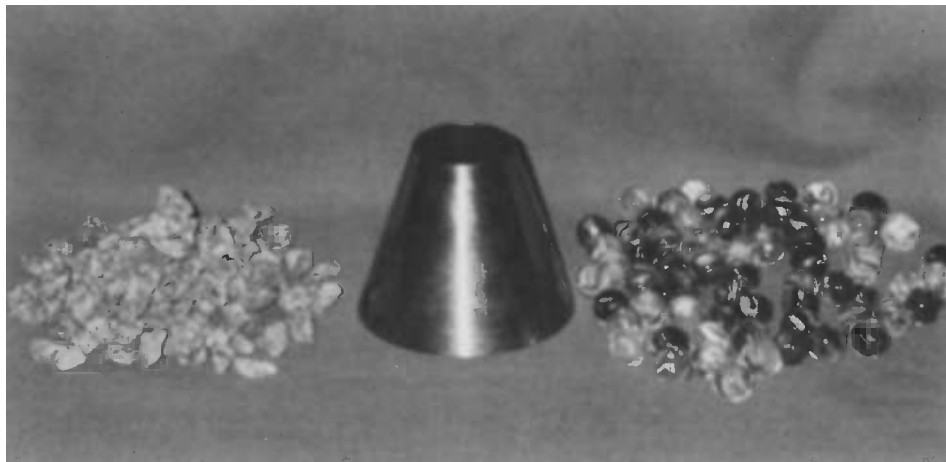
Fig. 1—Aggregate mobility affected by shape and surface texture.
