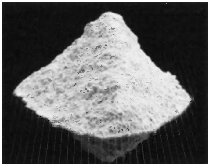
Fig. 6 —After grinding, the slag granules become slag cement.
