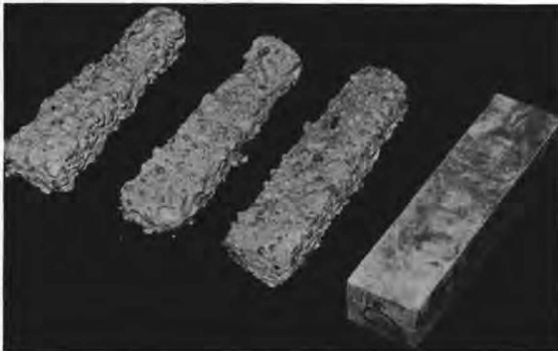
FIG. 1—Surface sloughing of durable concrete specimens frozen and thawed in water according to ASTM Method C 290. Three specimens on left were removed after 300 cycles of freezing and thawing. Specimen on right unfrozen.
