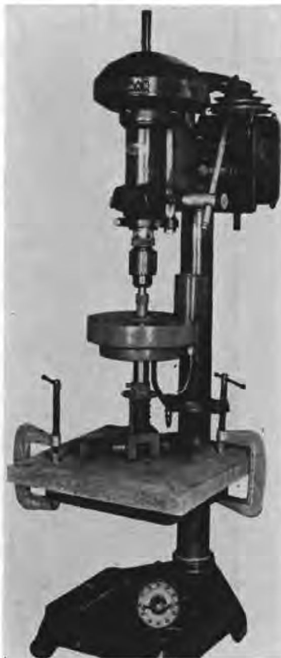
FIG. 3—Drill press operated dressing wheels.
