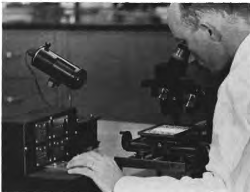
FIG. 3—Performing the petrographic examination of fine aggregate with stereoscopic microscope, mechanical stage, and tally counter.
