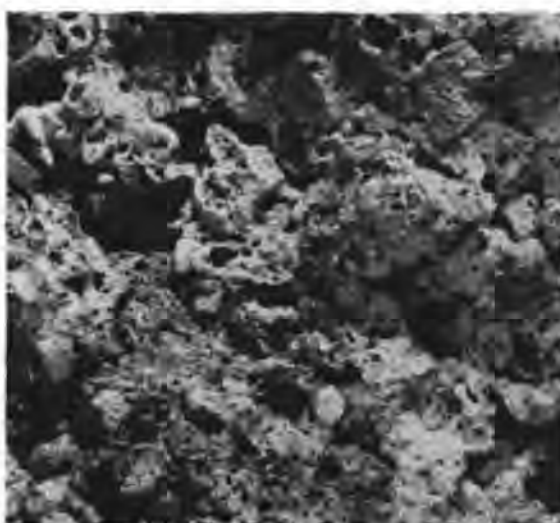
FIG. 2—Coal in sintered clay before crushing ( \times 2.7 ). Reduced one half for reproduction.
