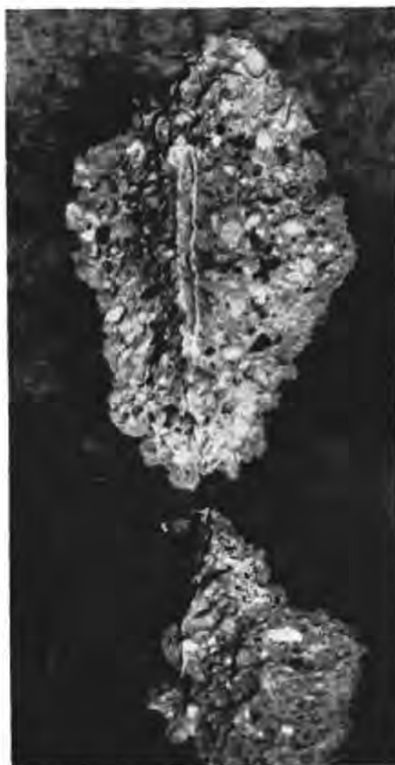
FIG. 1—Concrete spalled by corroding aluminum conduit (from Ref. 5).
