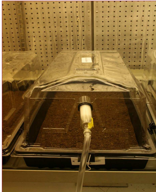
FIG. 2 Assembled closed dome system.
