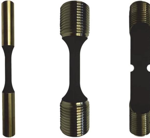
specimen surface and the TP as described in previous work [19]. A conventional air spray gun was used to apply the paint to a thickness of approximately 20–25  $\mu\text{m}$ . The paint was then air dried and cured in a furnace at 300°C for 1 h. A scanning electron microscope (SEM) image of the thickness of the HE23 TP coating on the surface of a test piece is given in Fig. 3.
