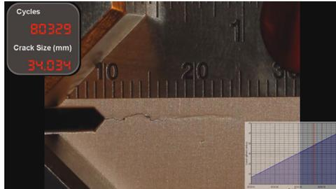
growth test, it is apparent that this is due to the well-known crack front bowing due to plane strain conditions in the bulk of this specimen.
