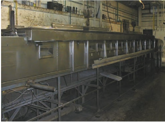
FIG. 1— Photograph of Exterior of Steiner Tunnel.
