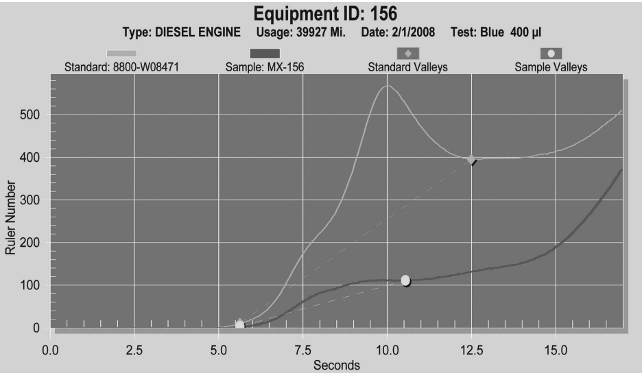
FIG. 7—Voltammograph from Unit 156, collected at 39,927 lube miles and 8.9% remaining antioxidants.
