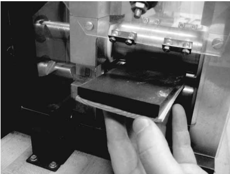
FIG. 4—Duplicates of the wood specimens are made using a die in the Technovate Rolling Mill (photo shows specimen going into the press).
