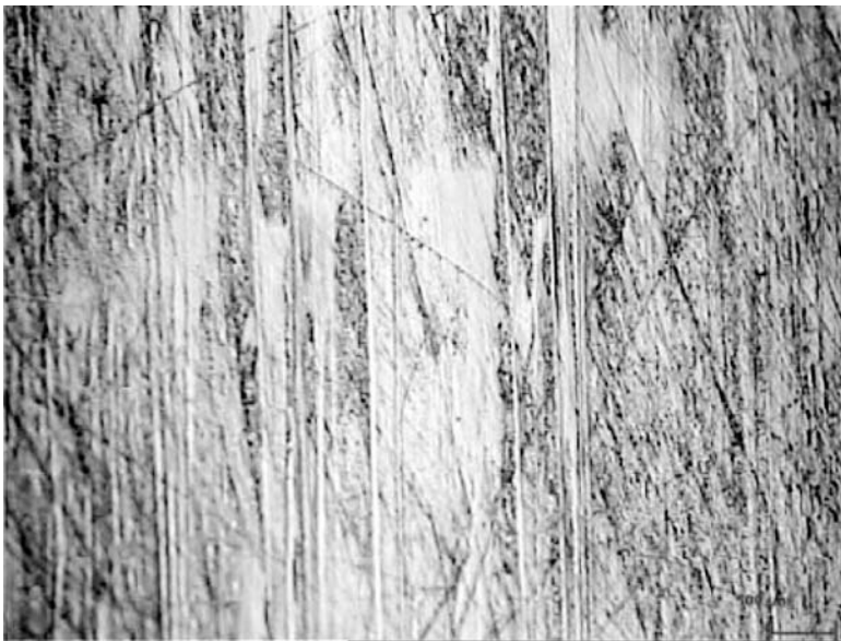
FIG. 8—Polished wear area of the femoral articulation of specimen PS3 (original magnification 100 \times ).
