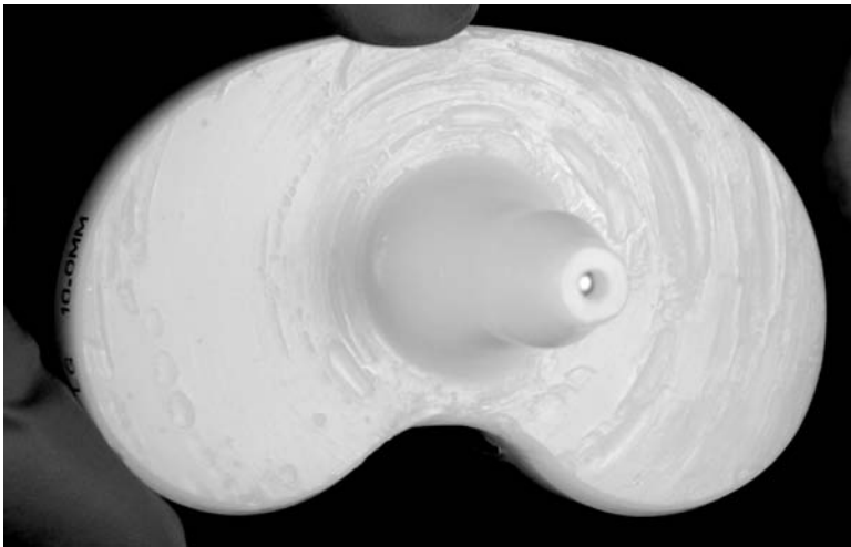
FIG. 7—A retrieved rotating platform shows moderate rotation surface damage after only 5.7 months in vivo. Wear penetration on this bearing was 0.013 mm, well below the average of 0.07 mm for the series.
