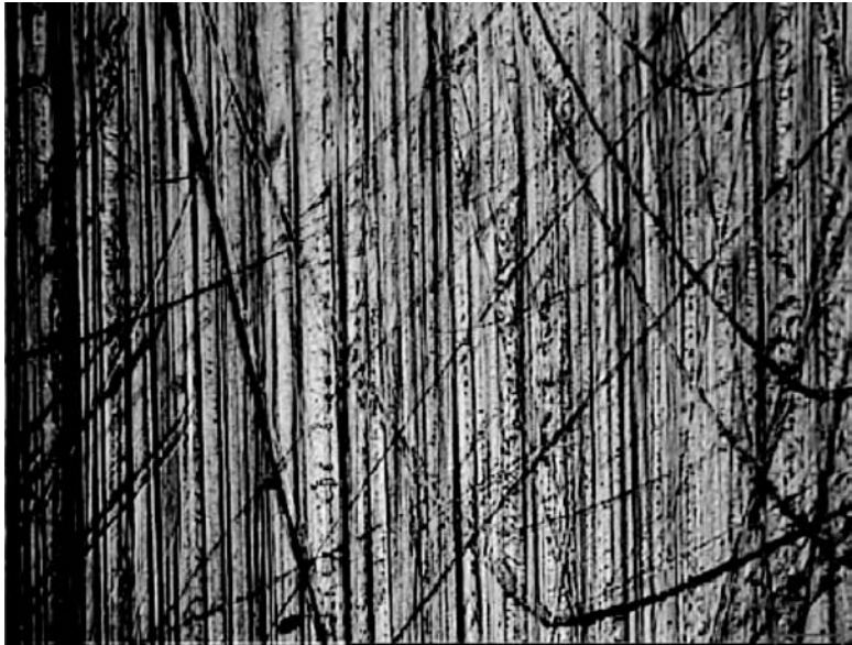
FIG. 9— Scratched wear area of the femoral articulation of specimen PS2 (original magnification 100 \times ).
