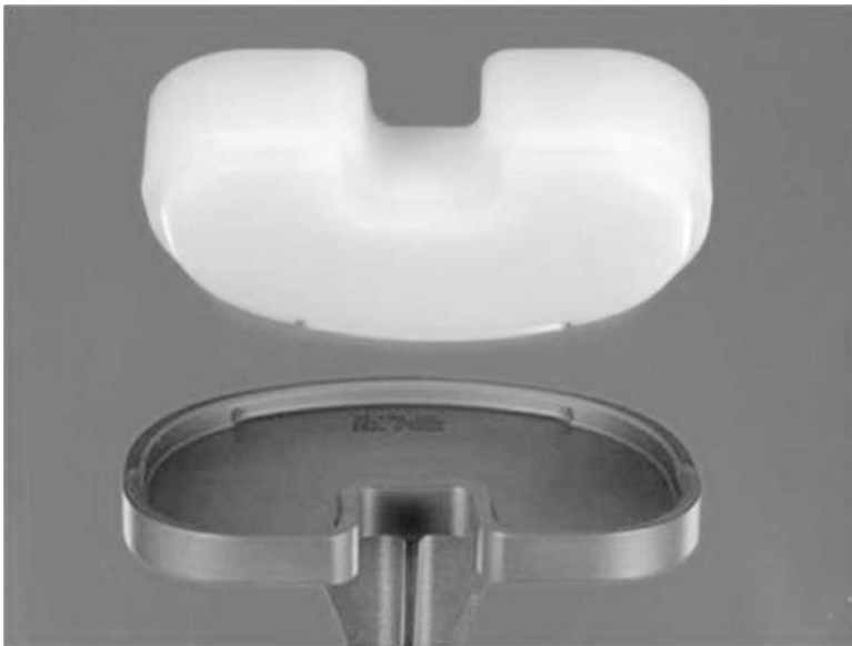
FIG. 8—PFC ® Fixed Bearing knee, which had a titanium alloy tibial tray with a grit-blasted surface. Relative motion of the UHMWPE bearing insert and the tray has been shown to cause increasing wear rate of the bearing with duration in vivo.
