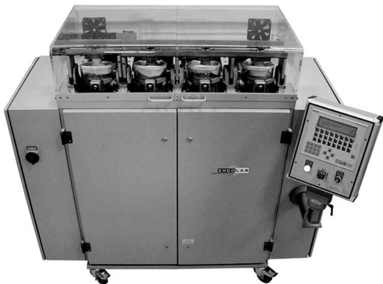
FIG. 2— Knee simulator at EndoLab/Germany. Force-control testing with soft tissue simulation. Loaded soak control is implemented on one of the four test stations.
