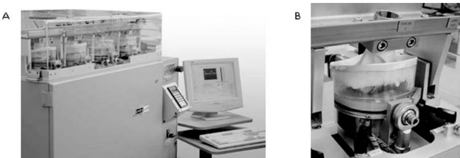
FIG. 1—Computer-controlled four-station knee simulator: (a) Provides a general view of the simulator while (b) showing a detailed view of one station (with the permission of Endolab).
