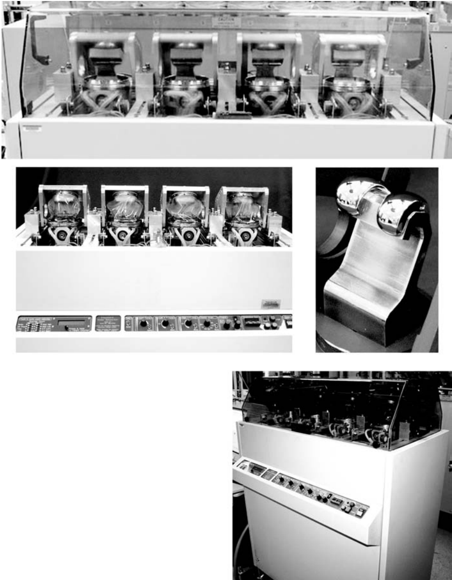
FIG. 1—One of the three knee simulators at the University of Nebraska Medical Center. The simulator has 4 test stations that are servo-electrically and pneumatically driven. Loaded-soak controls are implemented on a separate, dedicated external machine. Middle right: Example flexion bracket custom made for optimum sagittal plane alignment of an individual implant. Top: Large stainless steel tibial component dishes for high range TKR motion. Bottom: Serum bags used in some tests to increase the amount of lubricant per station with some TKR designs.
