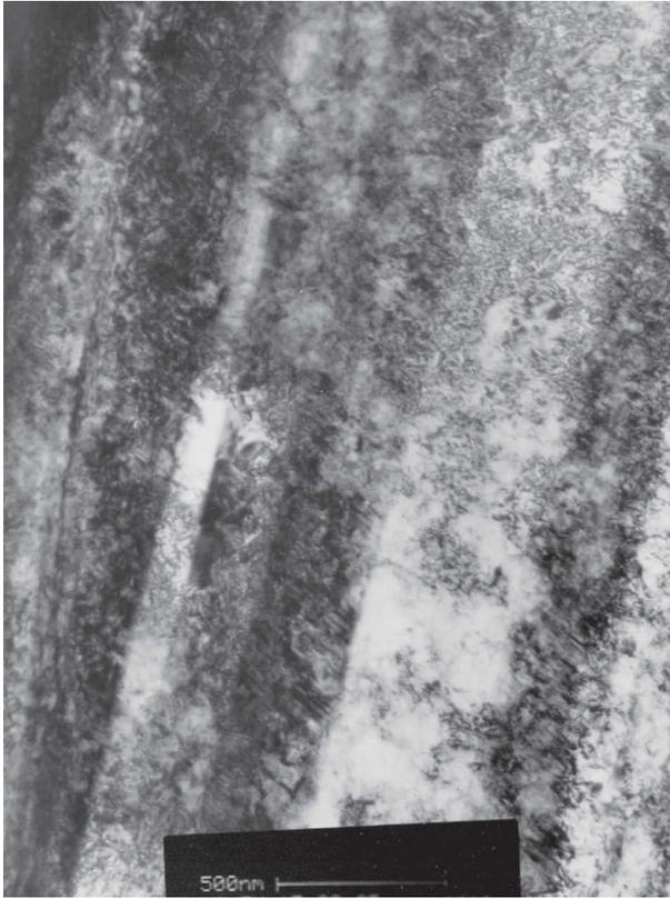
FIG. 3—CW structure of the unirradiated 316 stainless steel wrapper.
