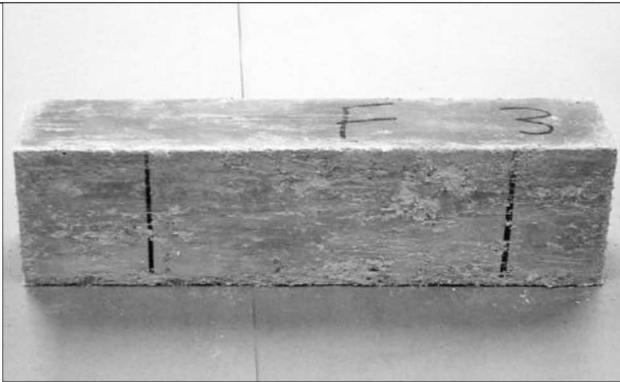
(b) ECC (with fiber) after 300 freezing and thawing cycles
