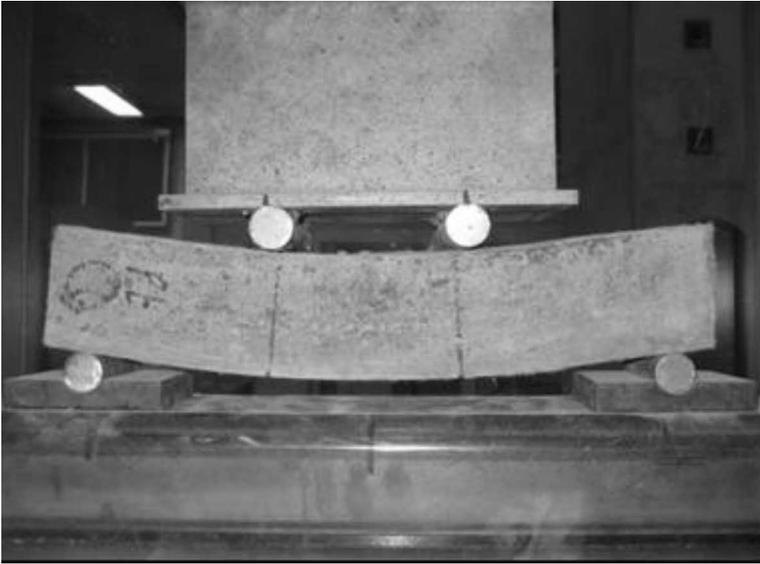
FIG. 2—Response of ECC beam after 300 freezing and thawing cycles under flexural loading.
