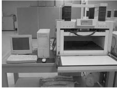
FIG. 1— Photograph of the heat-flow-meter apparatus.
