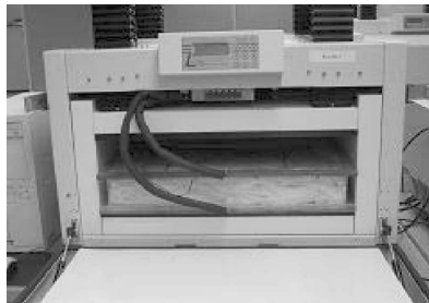
FIG. 3— Photograph of the test box positioned in the heat-flow-meter apparatus.
