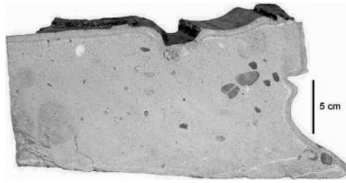
FIG. 7—Cross section of a typical Roman cement cast mortar with a very low amount of aggregate and some large gravels; the rim has residues of glue or oil steaming from the mold or the release agent, respectively. The long side of the element is about 30 cm (photo: Chr. Gurtner).
