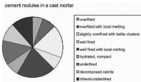
FIG. 11—Relative amount of the various types of cement relicts in the binder of a single sample from a typical historic Roman cement cast mortar, analyzed by thin-section microscopy combined with SEM/EDX; total amount of phenograins: 69. All types of phenograins are represented in the mortar at nearly equal proportions. (See color insert for color version of this figure).
