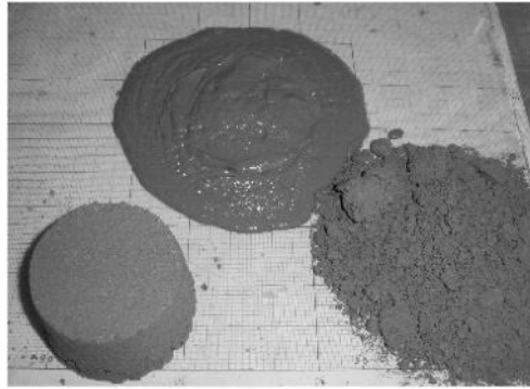
FIG. 5—Natural cement at 0.3 water-cement ratio. The incoherent mix (lower right) is readily compacted (lower left), but addition of a commercial superplasticizer results in high fluidity (center), facilitating use for stucco and poured-in-place concrete without altering water-cement ratio or reducing strength.
