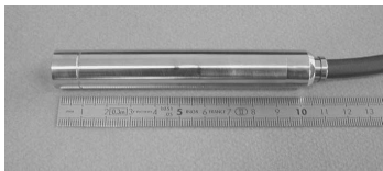
FIG. 4— HgI_2 detector assembly.
