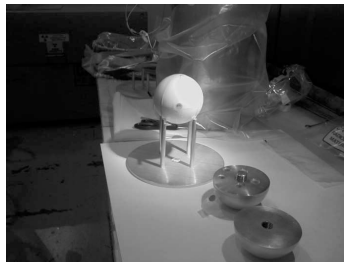
FIG. 2—10.16 cm diameter spheres with standoff for dosimetry bucket.
