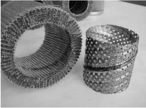
FIG. 15—The spiral construction of the center core and the contacting line on the internal surface of the fiber part.
