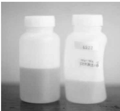
FIG. 23—Comparison of a plastic bottle with oil heated at 80^\circ\text{C} for six months (left) and the one with oil filtered for 30 days.
