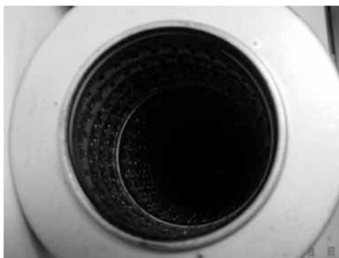
FIG. 14—The internal surface of the filter center core metal.
