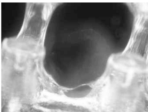
FIG. 19— Damaged nylon net adjacent to the spiral of the center core.
