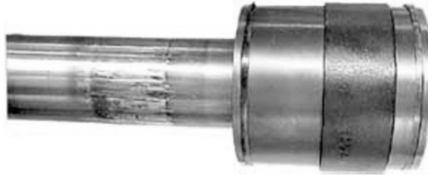
FIG. 1—Varnish formation on inlet guide vane (IGV) valve from a gas turbine.
