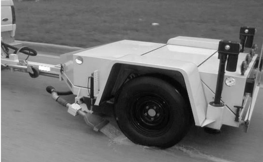
FIG. 1—Typical FDOT pavement friction testing unit performing a test.
