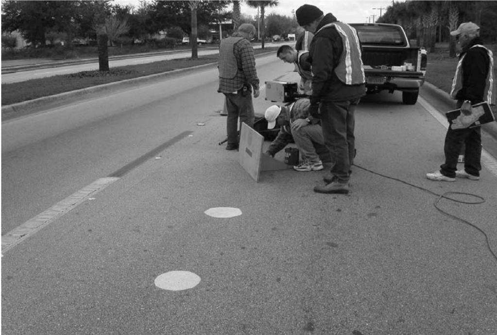
FIG. 5—Sand patch testing (ASTM E 965) within the wheel lock-up zone of a typical FDOT calibration test section.
