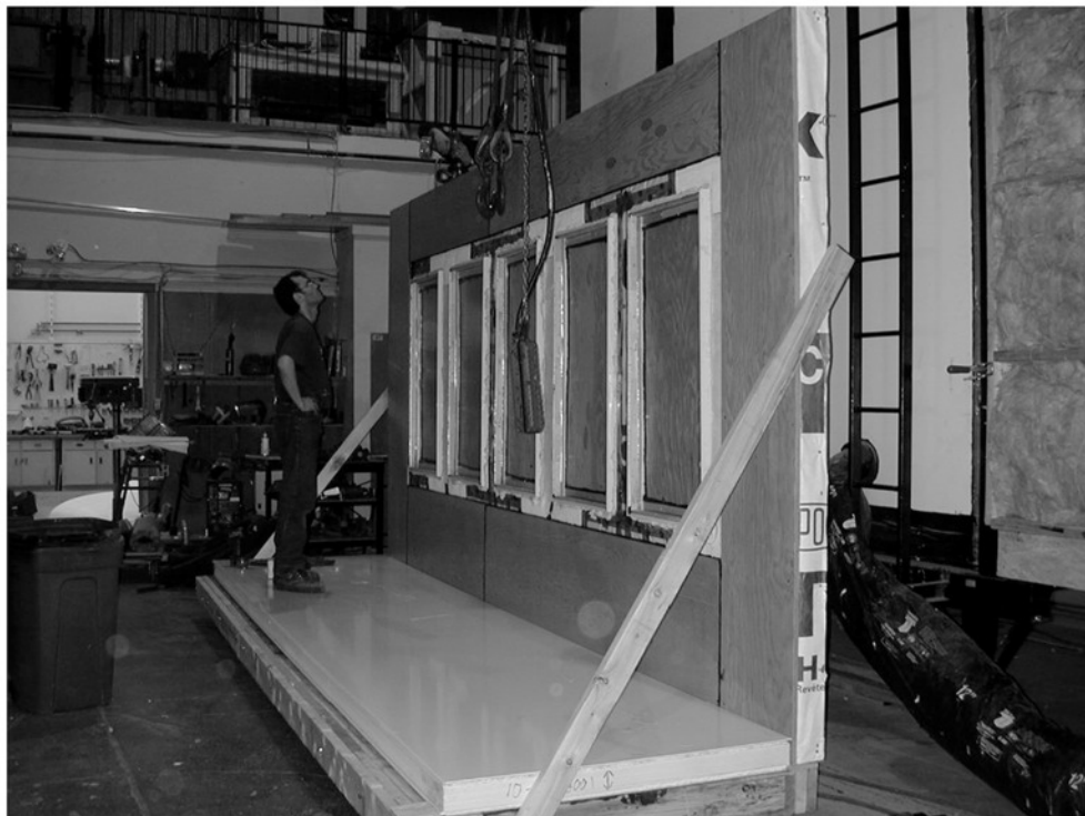
FIG. 4—Wall system being lifted into place on the conditioning chamber. The chamber can test air leakage, apply water spray, and temperature cycling.
