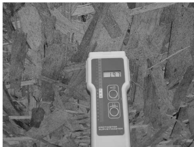
FIG. 4— OSB with an unadjusted moisture meter reading of 19.7 %.
