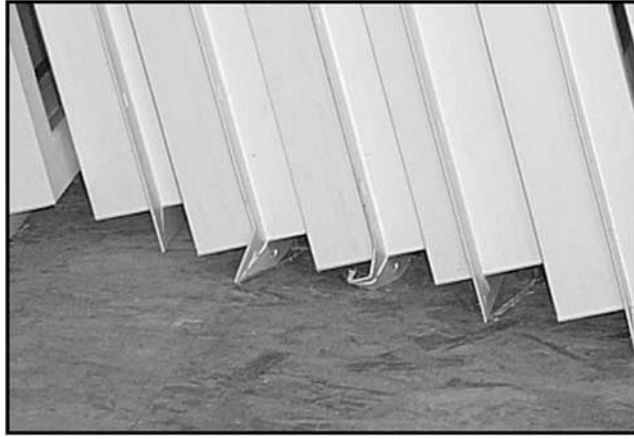
FIG. 26— Damage to window flanges.
