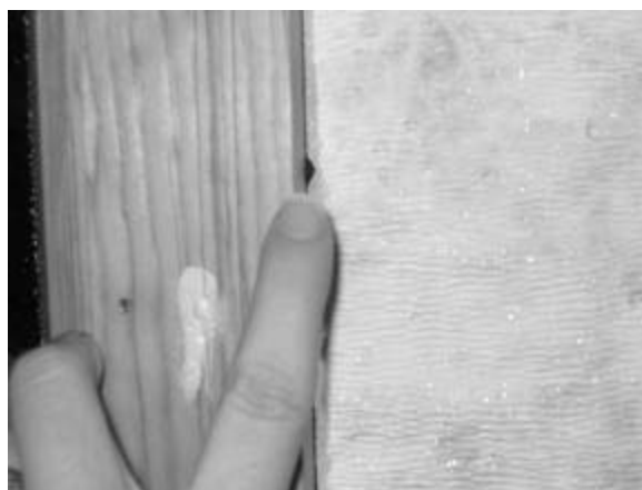
FIG. 8— Channel formation along jamb flashing after thermal cycling.
