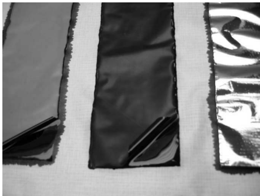
FIG. 11—Close-up of staining by modified-asphalt adhesive products after 70°C heat aging.
