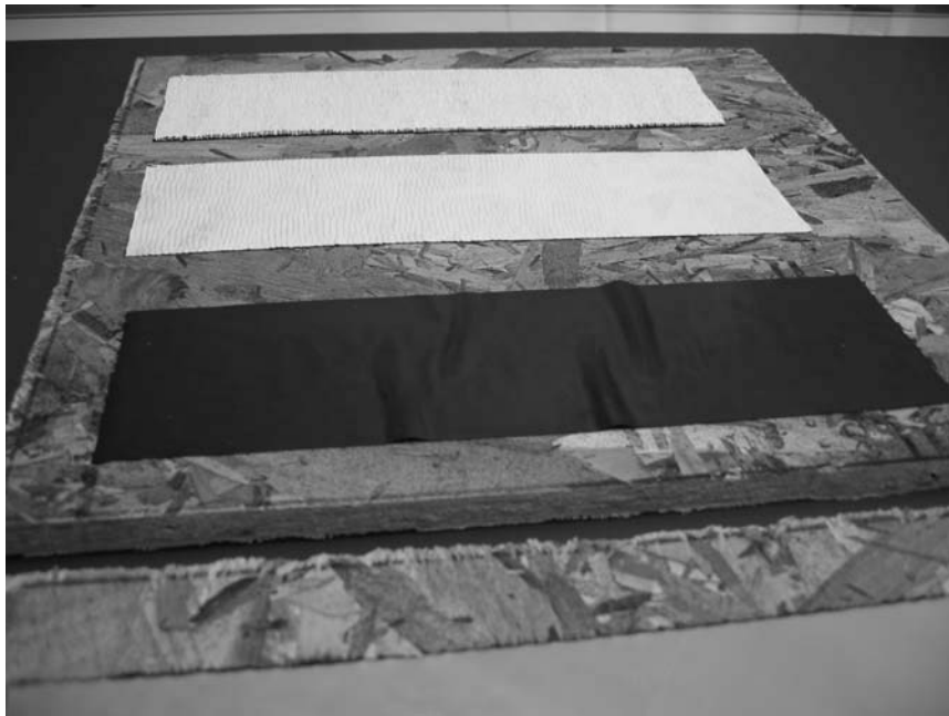
FIG. 9—Side-view of butyl-based adhesive products after thermal aging.
