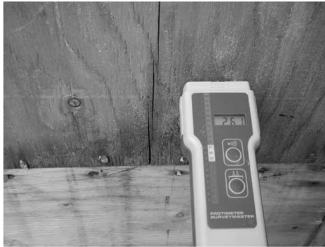
FIG. 2—Plywood sheathing showing an unadjusted reading from a moisture meter of 26.1 %.
