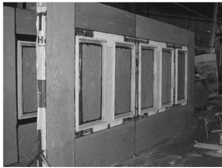
FIG. 2— A test wall containing five vinyl test window frames with the window blanked out using sealed plywood. Here the spun-bonded polyolefin house wrap is in position around window opening with foam products installed.
