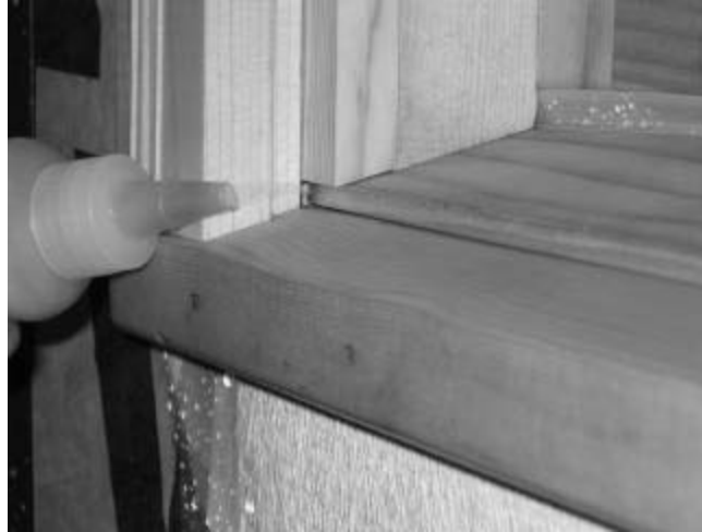
FIG. 3— Smoke flowing into a gap at the interface between the exterior sill and jamb brick molding illustrates air and water infiltration.
