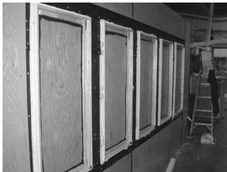
FIG. 3— A second wall unit setup with black building paper; plywood is installed in place of glazing.
