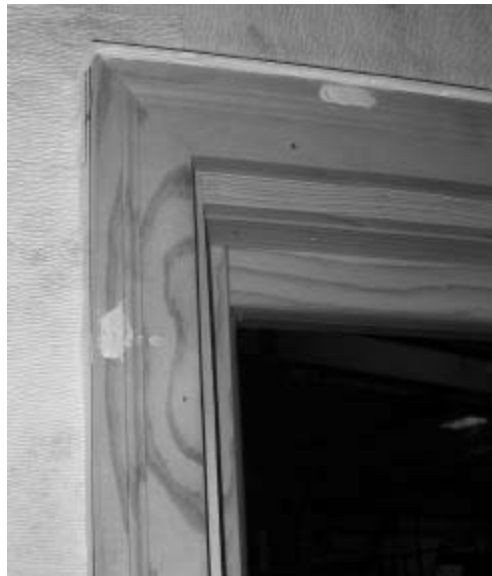
FIG. 4— Brick mold window miter joint before thermal cycling.
