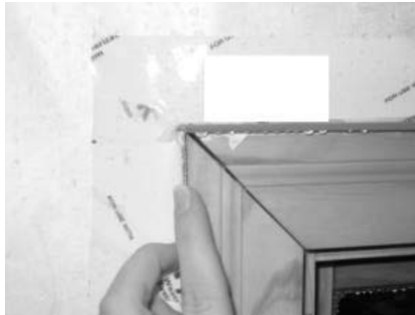
FIG. 5— Brick mold window miter joint after thermal cycling.
