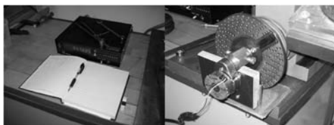
FIG. 4—Motor and digital device for measuring the angle of the tilting table.
