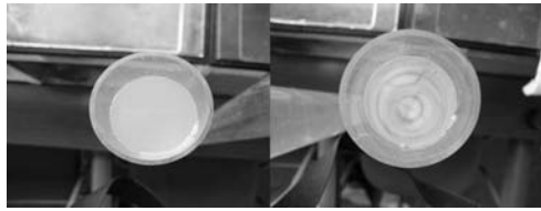
FIG. 4—Differences in transparency between pumped and filtered seawater.
