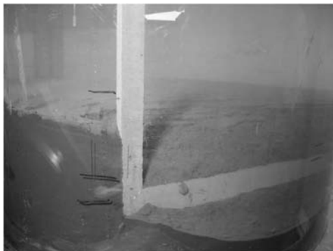
FIG. 11—Slope in sediment after standing for 24 h.
