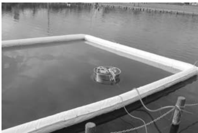
FIG. 12—Purification experiment using a small-sized filtration system.
