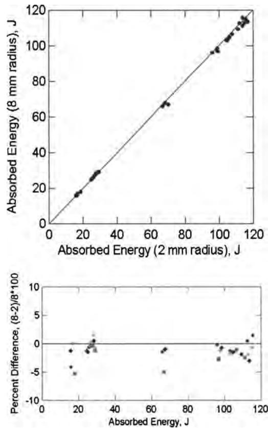
FIG. 4—A comparison of data for 8 and 2 mm striker geometries gathered by use of reference impact pendulums and type 4340 verification specimens. The upper plot (a) shows a general comparison, and the lower plot (b) shows the percent difference of the 8 and 2 mm striker data gathered on each machine (colors), for each set of verification specimens tested (the 2 mm data was subtracted from the 8 mm data, divided by the 8 mm data, and multiplied by 100).
