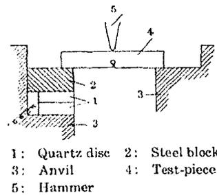
FIG. 10—Schematic of Watanabe's piezoelectric load cell arrangement [13].
