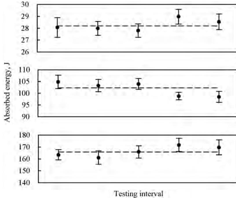
FIG. 2—Results of the routine check of the standard Charpy machine.
