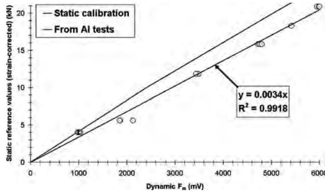
FIG. 4—Calibration curves obtained for one of the 8 mm strikers. The red line was obtained by applying the static calibration procedure using a flat support, as previously described.
