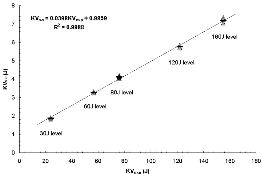
FIG. 3—Relationship between  $KV_{s-s}$  and  $KV_{exp}$  for the sub-size samples prepared from broken full-size specimens. Thick short lines indicate average values within energy levels.
