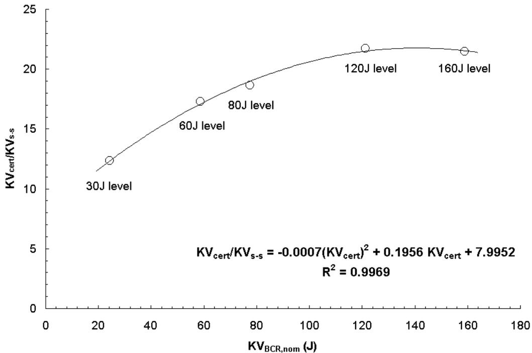
FIG. 6—Ratio between energies absorbed by full-size and sub-size specimens prepared from unbroken full-size samples.
