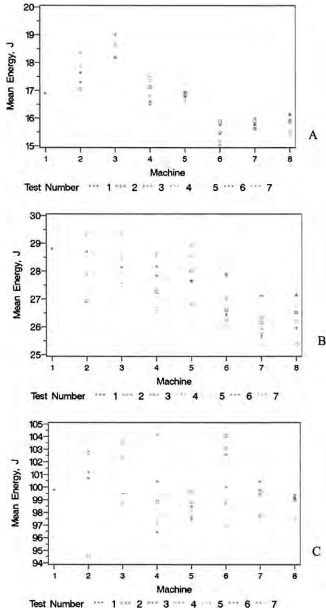
FIG. 3—The average energy of (a) low, (b) medium, and (c) high energy specimens is shown for each machine and test. Here the grouping of data for a given machine is most apparent. At low energy (a) the relative difference between machines and the lack of overlap for the data indicated clear differences due to the machines.
