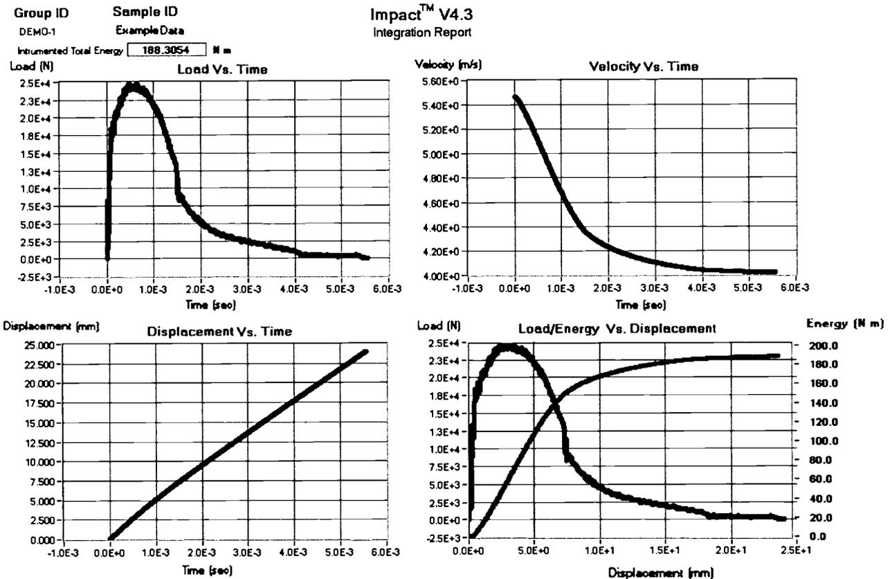
FIG. 2—The raw voltage-time signal has been converted to the force-time signal through the striker calibration. The force-time curve is integrated to give the velocity-time curve. The velocity-time curve is integrated to give the striker displacement-time curve. Finally, the force-displacement curve is integrated to give the energy absorbed by the test specimen.
