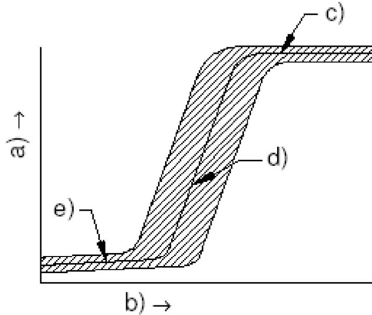
FIG. 1—Schematic diagram of the steel energy absorbed-temperature curve: a) absorbed energy, b) temperature, c) upper shelf zone, d) transition zone, e) lower shelf zone.
