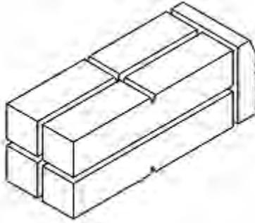
FIG. 2—Extraction of four KLST specimens from a broken full-size specimen half.
