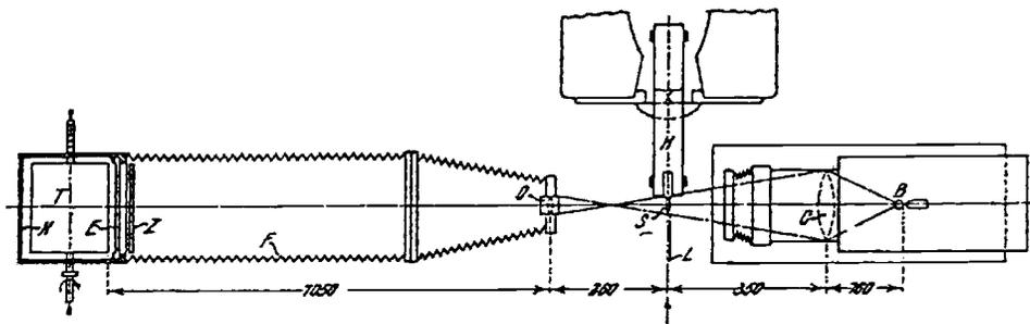
FIG. 8—Schematic of experimental arrangement of Korber et al. for measurement of hammer deflection at 4× magnification [7].
