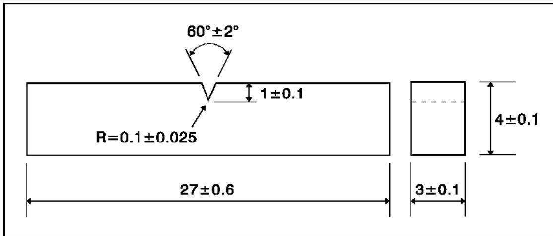
FIG. 1—Sub-size specimen of the KLST type used in this investigation (dimensions in mm).
