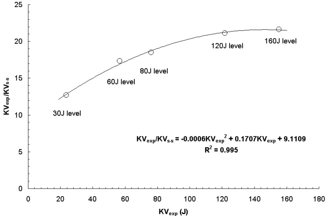
FIG. 4—Ratio between energies absorbed by full-size and sub-size specimens prepared from broken full-size specimens.
