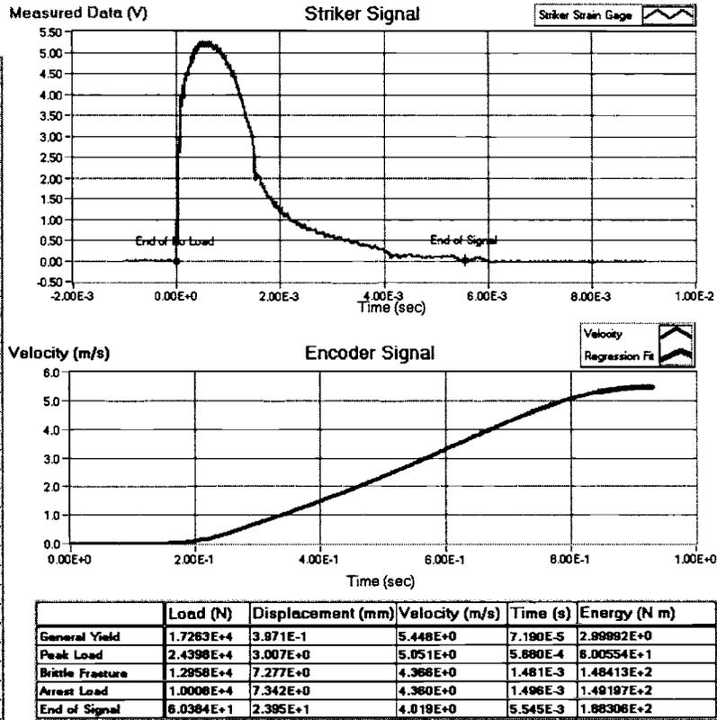
FIG. 1—Strain gage voltage-time signal obtained with a modern instrumented striker system. The lower plot shows the striker velocity from release up to impact.
