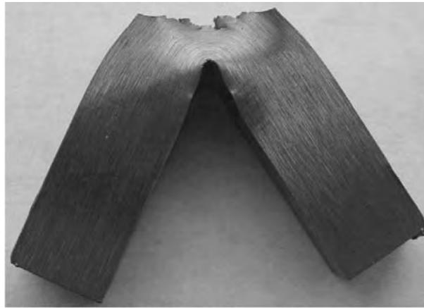
FIG. 3—The low carbon steel impact specimen impacted shown schematically.
