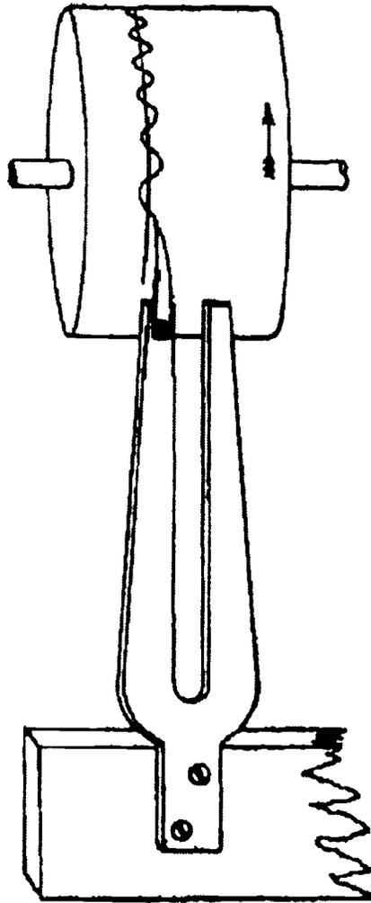
FIG. 5—Dunn's original tuning fork arrangement for time measurement [6].
