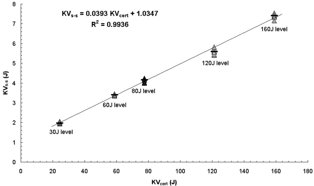
FIG. 5—Relationship between  $KV_{s-s}$  and  $KV_{BCR}$  for sub-size specimens prepared from unbroken full-size samples. Thick short lines indicate average values within energy levels.
