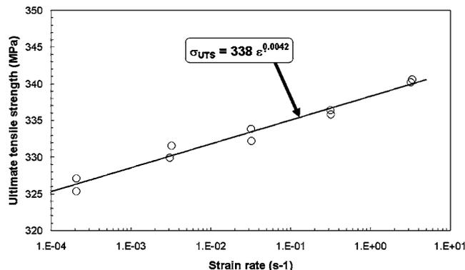
FIG. 2—Strain-rate sensitivity of the Al 6061-T651 alloy measured from tensile tests.
