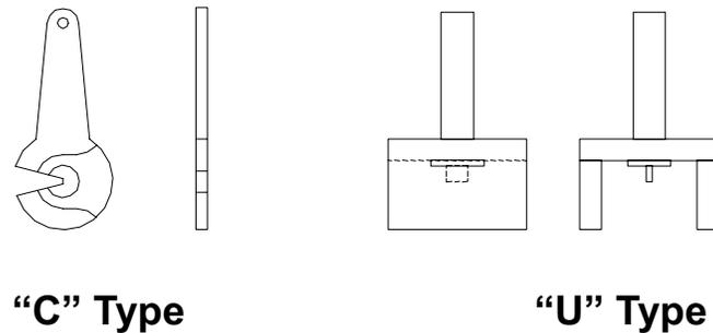
FIG. 1—Machine pendulum designs.
