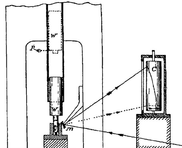
FIG. 4—Schematic showing Dunn's method for measuring deflection data by projection of light onto a revolving photographic film [6].
