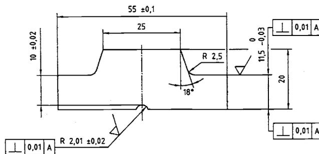
FIG. 1—Calibration support block suggested by the ISO 14556:2000 standard.
