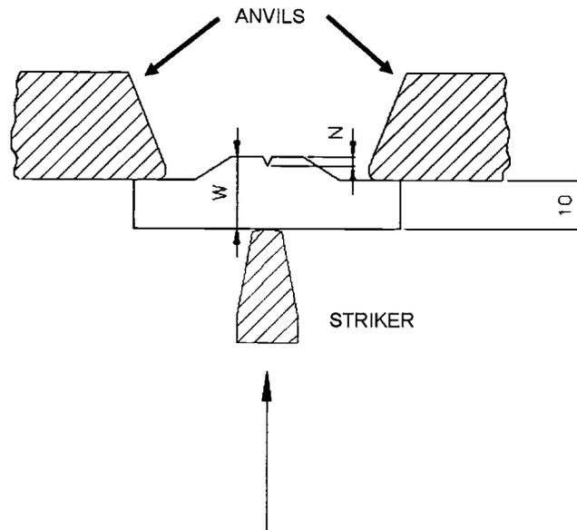
FIG. 3—Configuration for impact tests on modified Charpy specimens of Al alloy 6061-T651.
