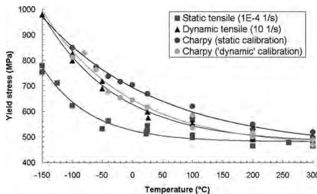
FIG. 5—Comparison of yield stresses measured from tensile and instrumented Charpy tests for one of the 2 mm strikers investigated; values corresponding to the “dynamic” calibration are in much better agreement with tensile data than those of the static calibration. Tensile and impact tests were performed on the 18MND5 RPV steel.
