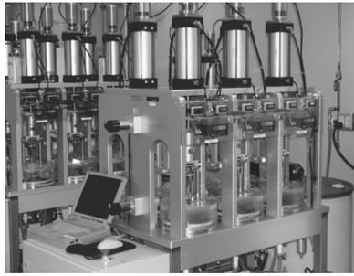
FIG. 2—Multi-station spine wear simulator.
