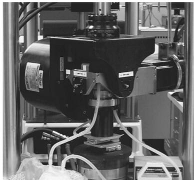
FIG. 3—Single-station spine wear simulator.
