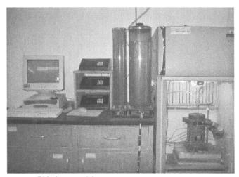
FIG. 3—Actual freeze-thaw/gas permeability test cell.
