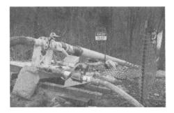
FIG. 7 - Ash/water mixing gun.
