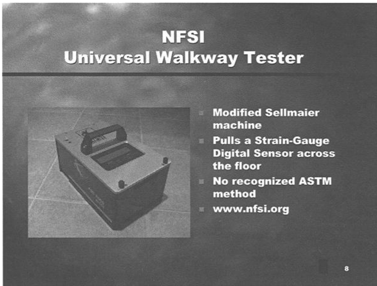
FIG. 7-The NFSI Universal Walkway Tester
