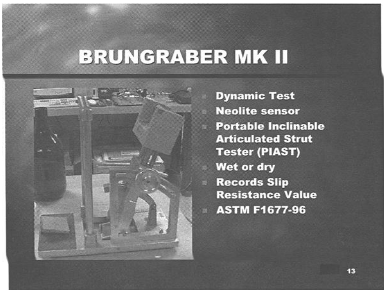
FIG. 11-The Brungraber Mk II Portable Inclined Articulated Strut Tribometer
