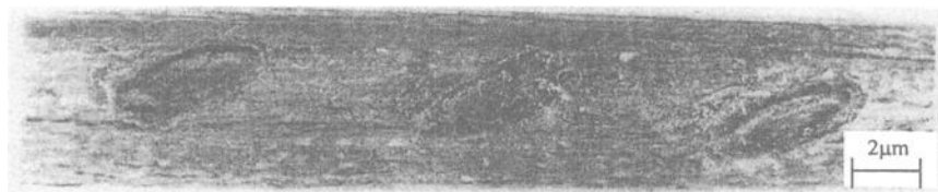
Figure 4 – Wire from rope with fretting marks from a trellis contact
