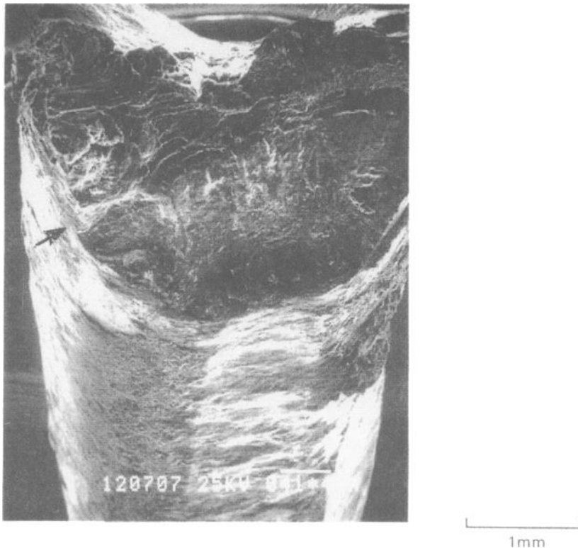
Figure 15 Low power SEM micrograph of cracked strand broken open to reveal fracture surface (final position of fatigue crack tip arrowed)
