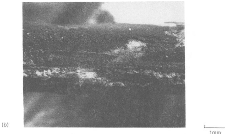
(b) development of flat close to edge of clamp
