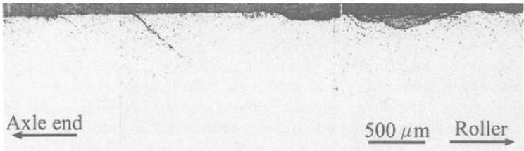
Figure 7—Sectional View of Microcracks
