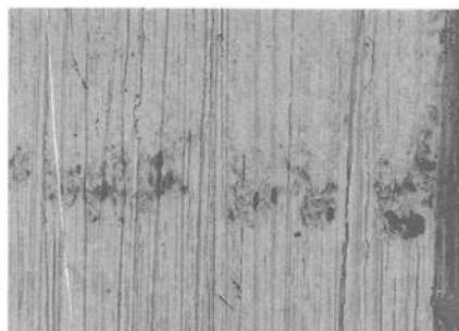
Figure 7 — Non-crack wear debris for 100%-of-life at 620 MPa clamping stress. ( N_f = 22\,600\,000 cycles)
