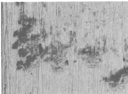
Figure 6 — Wear debris for 100%-of-life at 200 MPa clamping stress. ( N_f = 144\,000\,000 cycles)
