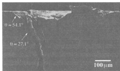
Figure 2 - Micrograph of primary fretting fatigue cracks in PH 13-8 Mo stainless steel.
