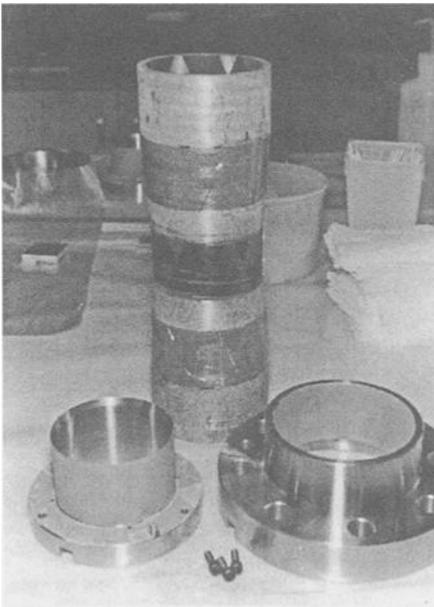
Figure 1—Multi-axial composite tube.
