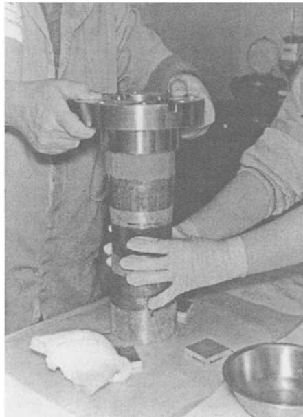
Figure 2—Bonding of stainless steel ends.
