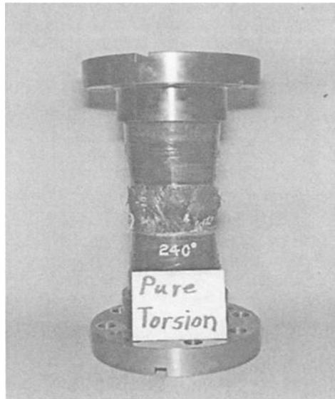
Figure 9—Failed tube loaded by torsion only.
