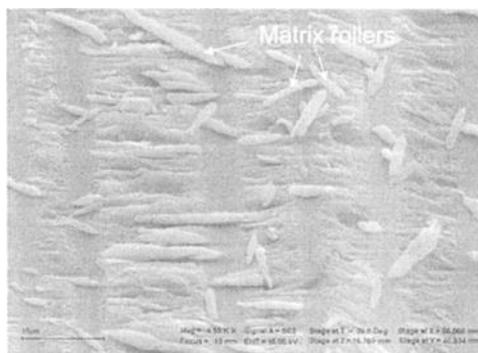
Figure 2 – Matrix rollers generated under Mode II fatigue loading ( $\times 4550$ ).
