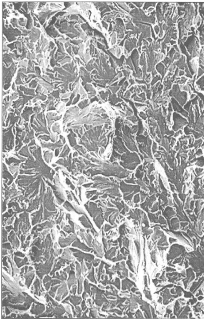
Figure 8. Scanning electron fractograph of as-received modified A302B steel Charpy impact specimen following irradiation at 288°C to 1 \times 10^{19} n/cm 2 .
