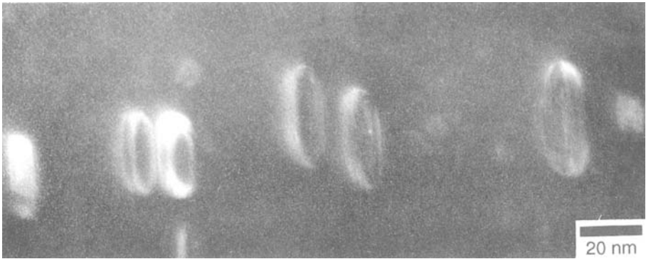
Figure 6 — Copper precipitates inclined to the specimen surface in Fe-0.6Cu aged at 500°C for 1000 h. The contrast is produced by strain field around the precipitates, indicating clearly that copper precipitate is of plate-type.
