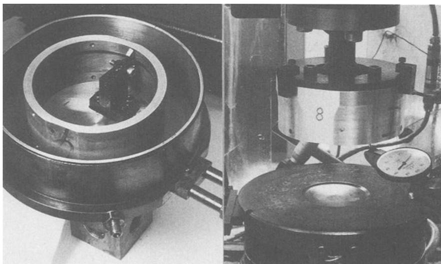
*Figure 2: Cylinder liner segment and piston ring contact situation (left figure: samples in the oil bath container; right figure: Arrangement for adjusting the rotating sample)*
