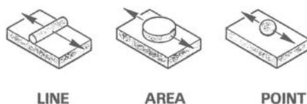
Figure 10 - Illustration of the tribo-contact conformity of various commonly used bench tests.
