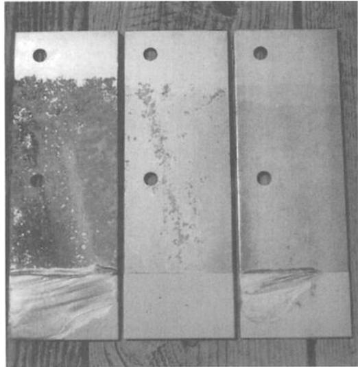
Figure 4 - Examples of crevice corrosion which developed under coating on sheet specimens. Shown N08367 with 20% of original mill surface coated
