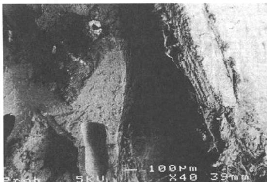
Figure 3 - SEM picture of a freeze fractured surface of a composite-membrane with a middle layer composed of poly (*L*-lactide-co-*D,L*-lactide) and coral hydroxyapatite particles (300-500  $\mu\text{m}$ ) in a 80/ 20 weight ratio.
