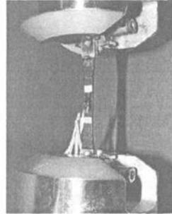
a) Schematic of the in-plane tensile test    b) Example of an in-plane tensile test
