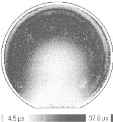
Figure 4. - Lifetime map of an  $n/n^+$  epi wafer (epi thickness  $17.5 \mu\text{m}$ , epi resistivity  $0.59 \Omega\text{cm}$ , substrate resistivity  $0.015 \Omega\text{cm}$ ) after the deposition of  $500 \mu\text{C}/\text{cm}^2$  positive charge.
